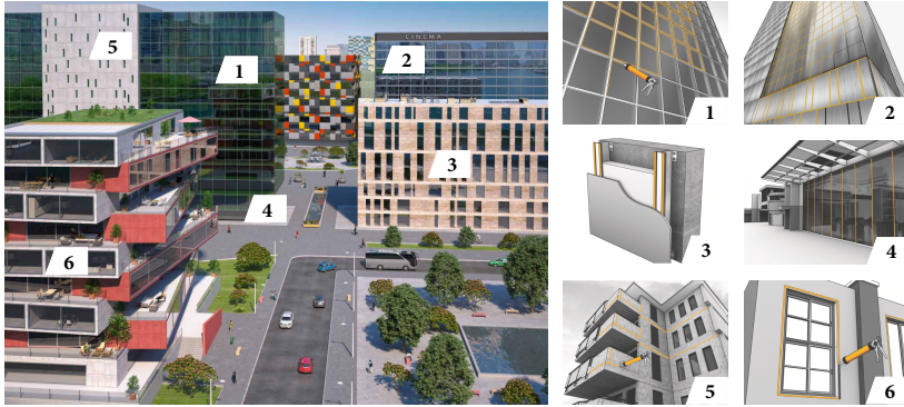
Fig. 1.2 Use of adhesives in facades. 1 Glass–glass joints, 2 glass–metal joints, 3 facade panel fixings, 4 translucent joints, 5 natural stone and concrete joints, 6 sealings (Sika Services AG, 2019a).
