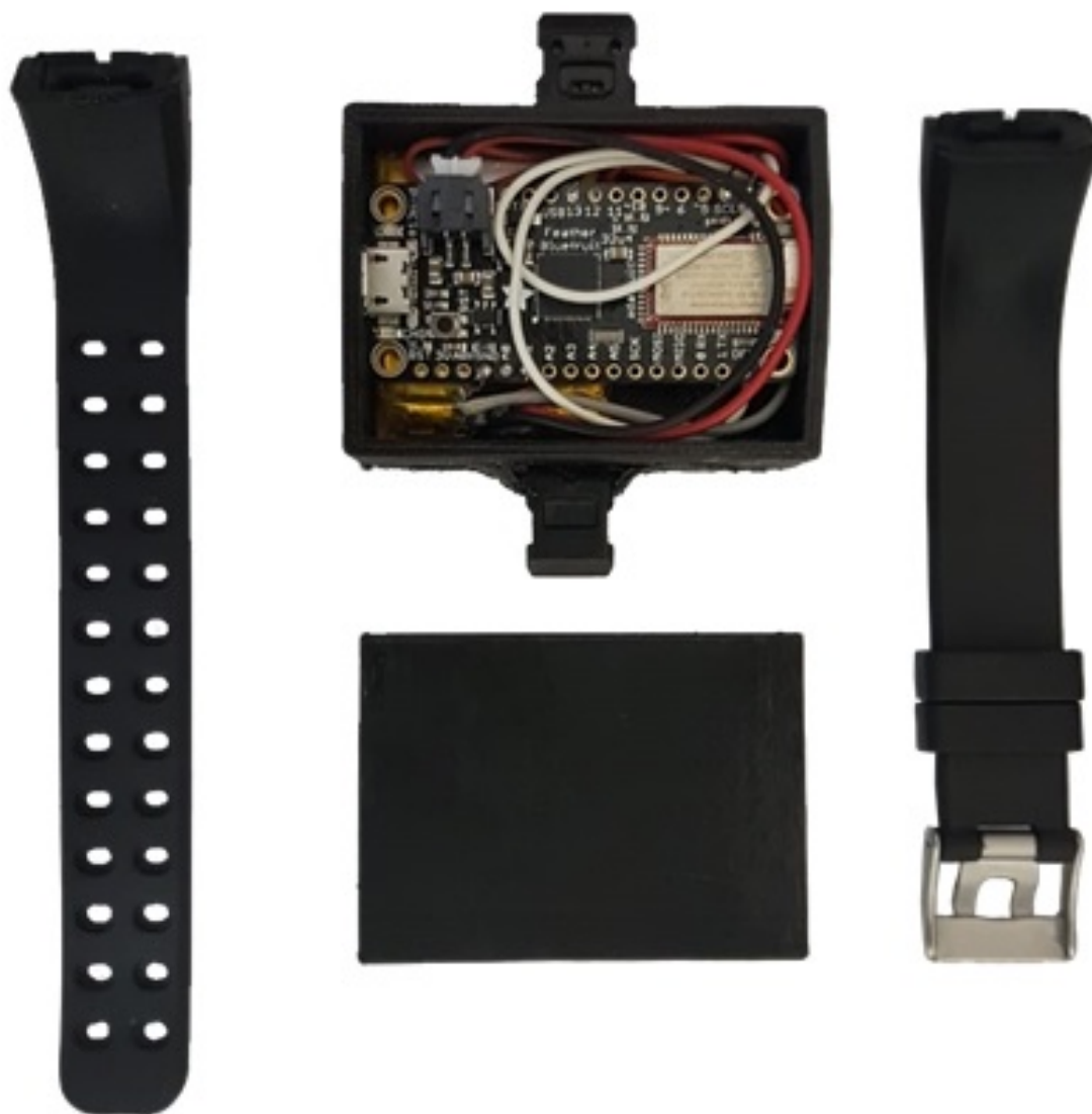
Figure 3. Prototype of the self-designed photoplethysmography sensor device.
