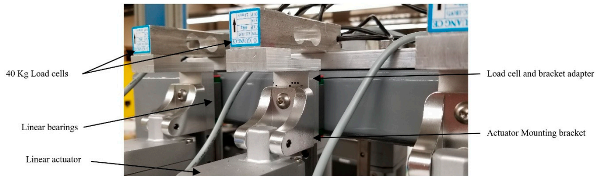
Figure 7. Linear actuator assembly.
