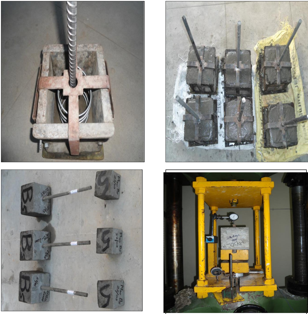
Figure 1. Arrangement for casting and testing of pull-out specimens
