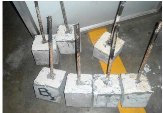
Figure 6. HYSD parallel and diamond rib rebar failure
