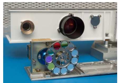
Artist's conception of ESA's ExoMars rover with PanCam on top of the mast, flight model of ExoMars Panoramic Camera „PanCam“, including DLR's HRC
