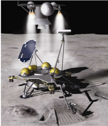
Artist's conception of the MoonRise lander concept with PanCam/MCI on top of the lander's mast.
