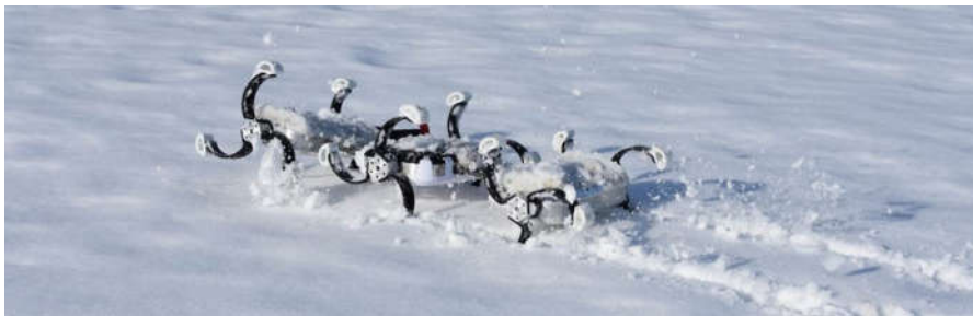
Small 10-30kg scale agile scouting rover for extreme terrain and planetary caves) based on rimless wheels
