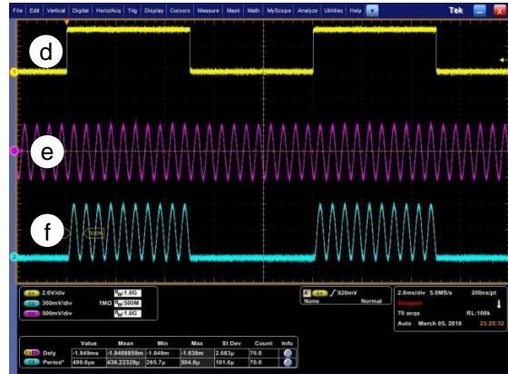
Fig. 9. Oscilloscope of (d) TTL gate input signal, (e) sine modulation signal and (f) measured light flux. LED current 10 A max and offset 0.53 V
