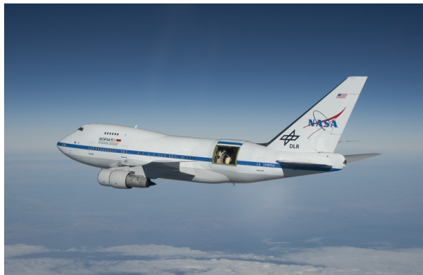
Figure 1.13: SOFIA airborne telescope during flight. Credit: NASA/Jim Ross.
