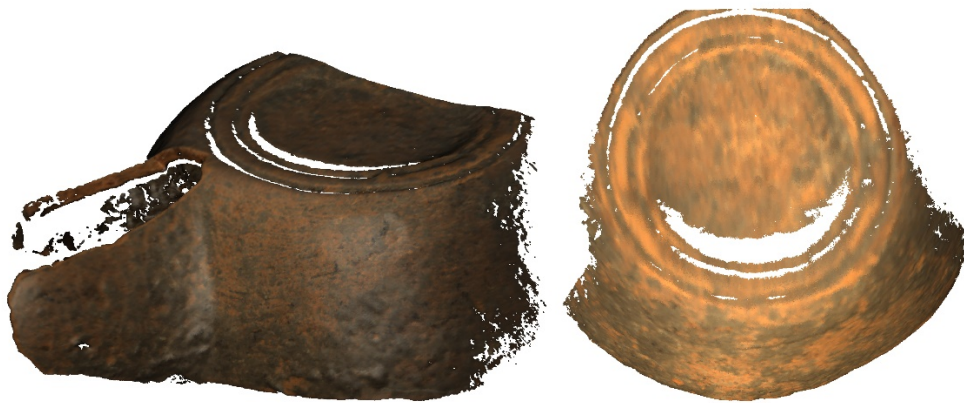
Figure 4.9: Poorly illuminated and blurry point clouds
