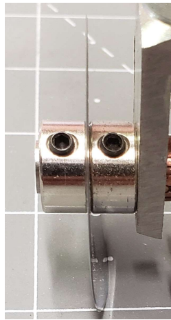
Figure 24: Bending of cutter due to excessive cutting pressure
