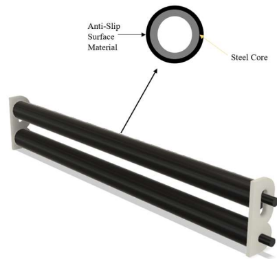
Figure 13: Cardboard feeder design decision
