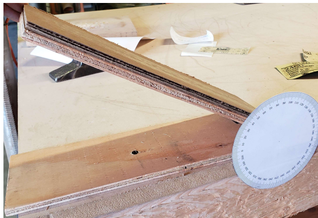
Figure 22: Experimental apparatus used to find the coefficients of friction
