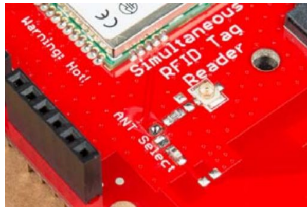
Figure 7: RFID Reader Antenna Select Solder Jump
