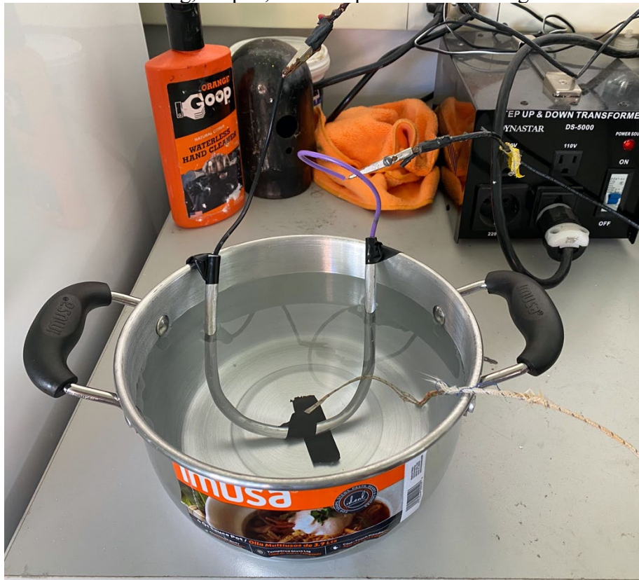
Figure L.2 Diode Immersion Heater Test Setup
