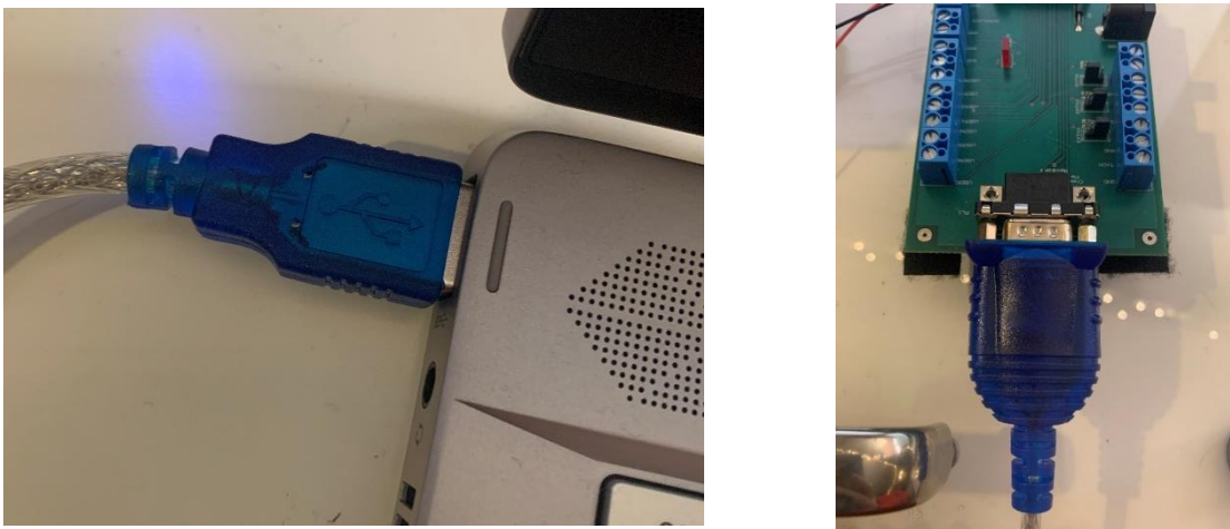
Figure 22. USB connection to the computer (pictured on the left) and the RS-232 Connection to the breakout board (pictured on the right)
