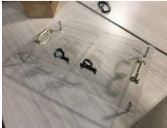
Figure 15. Handles, Bolts, Pump/O 2 Sensors Mounted
