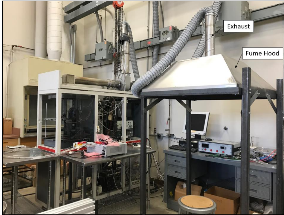
Figure 4: Oxygen Consumption Calorimeter in the Combustion Lab
