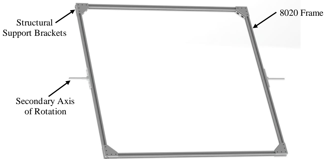
Figure 10. Inner Ring Subsystem on Structural Prototype
