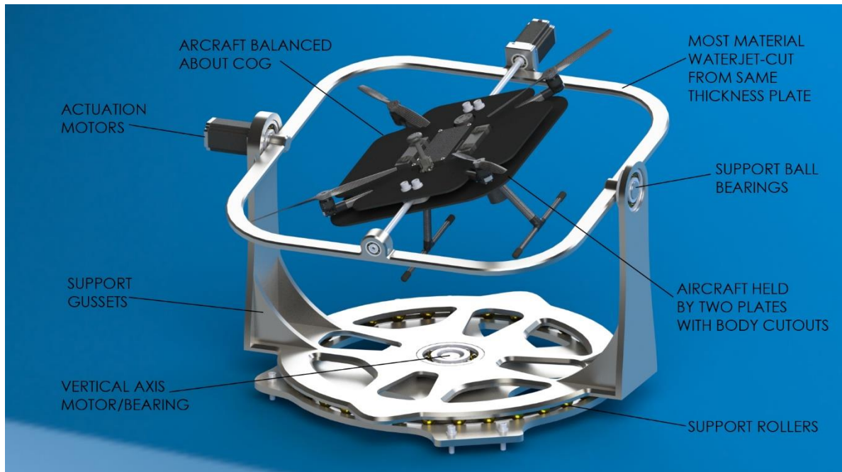
Figure 6. Isometric concept CAD model of gyroscope device
