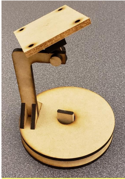
Figure 5. Concept prototype for turntable arm, laser cut from MDF
