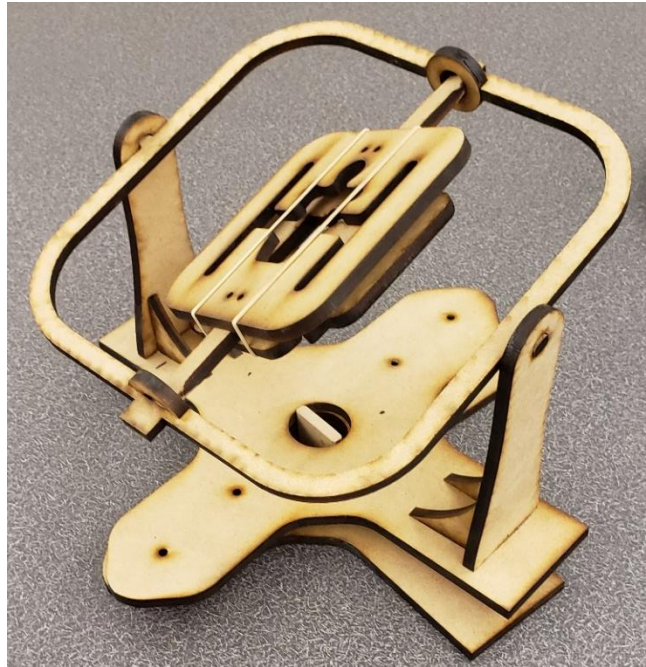
Figure 4. Concept prototype for the gyroscopic design, laser cut from MDF
