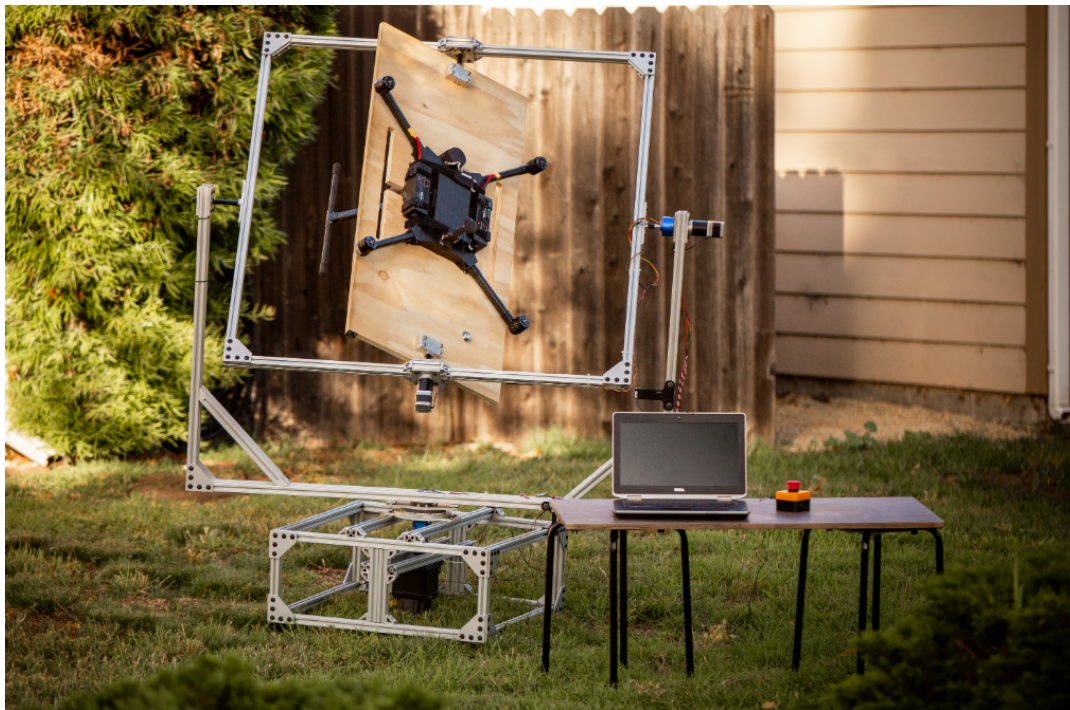
Figure 3: Overall Setup of Calibration System
