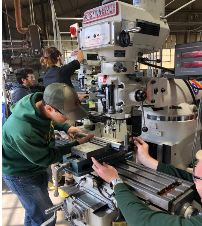
Figure 4. Setup on mill to cut slots into crank arms.
