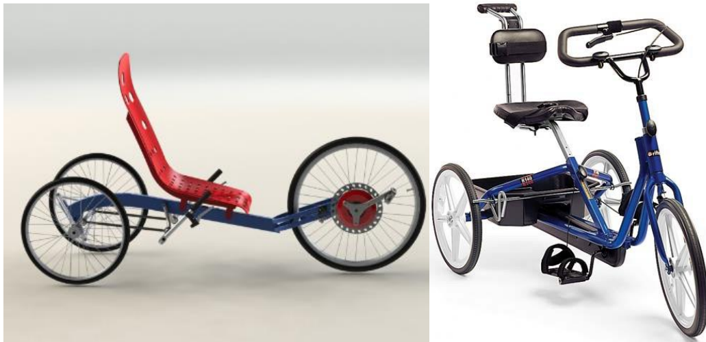
Figure 1. Right, adjustable open seating. Left, lean-to-steer mechanisms.
