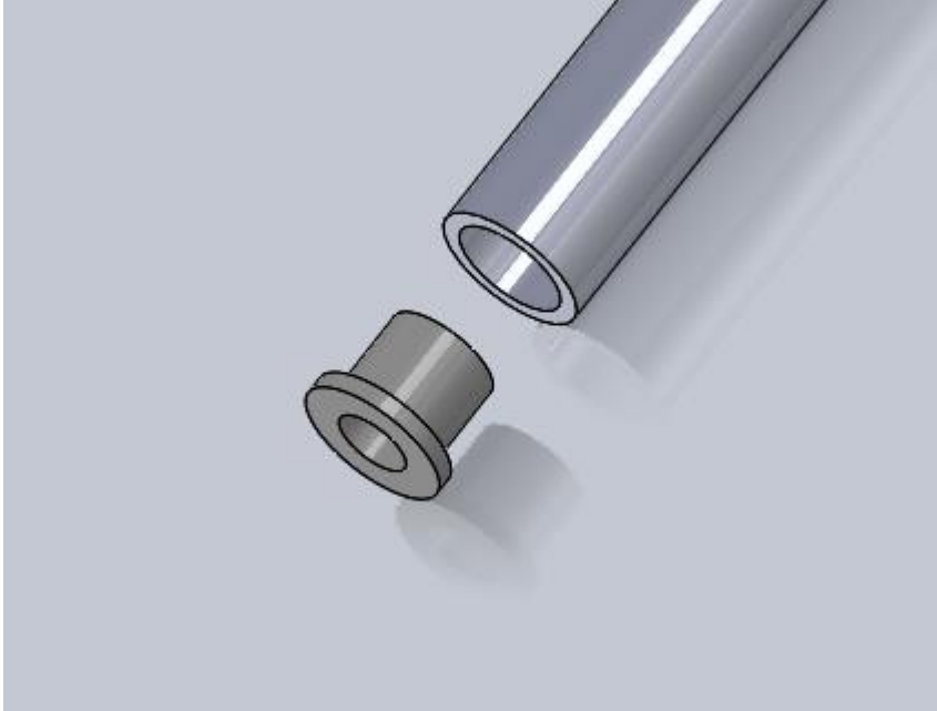
Figure 13. Close-up of top hat bearing (left) and steering shaft (right)
