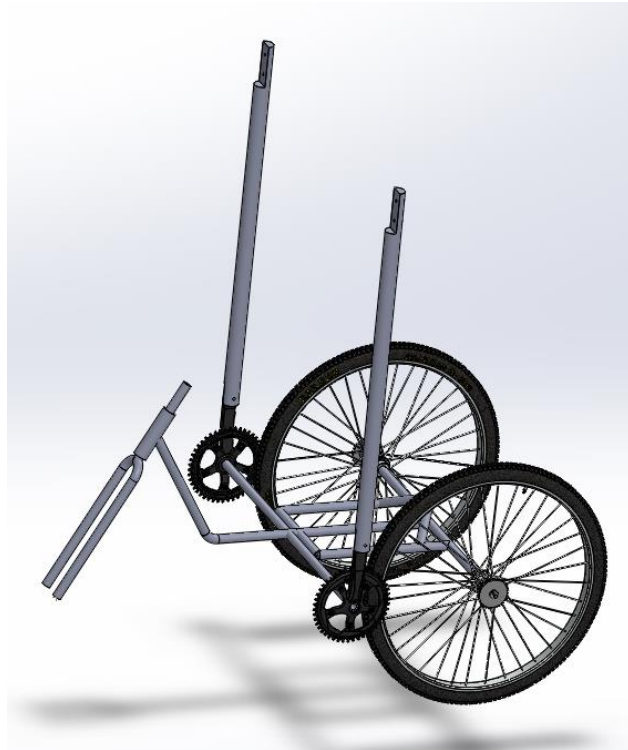
Figure 7. Crank arm and sprocket orientation once installed.
