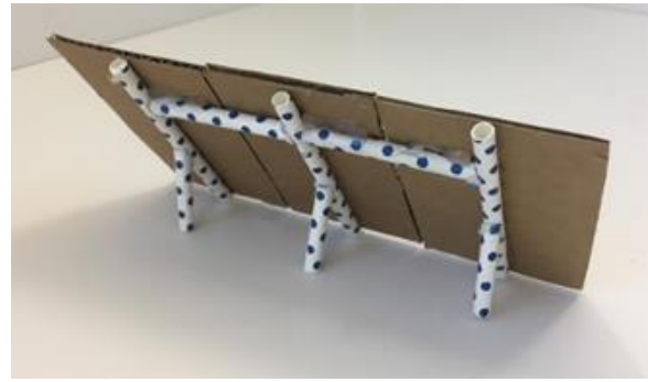
Figure 25. Fixed stand with three vertical bars and two horizontal bars holding three, same sized panels at a designated angle. This model only represents a way to fasten the panels down and does not solve the tilt issue.
