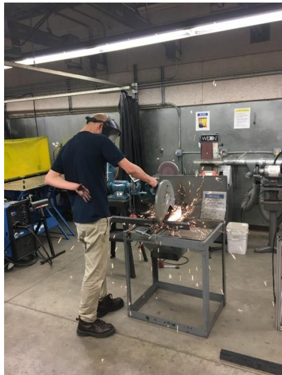
Figure 17. Cutting the Angles for the A-frame Leg Using an Abrasive Cutting Saw.
