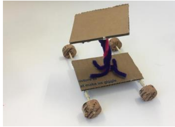
Figure 21. A concept model design for azimuth angle. The wheel design allows the mount to rotate and eliminates the need of another axis.
