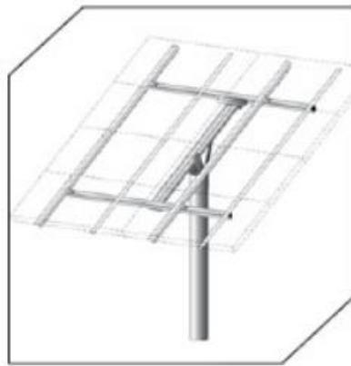
Figure 3: Top pole mount with multiple panels fastened to it [2].
