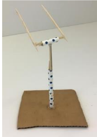
Figure 29. A concept model mount that has an azimuth angle adjuster at the top perpendicular joint, the two-stick member inside the vertical straw allowing for rotational adjustment, and the double prong stick to fasten the solar panels to.
