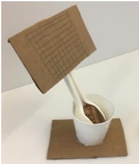
Figure 26. A concept model that shows the bottom point of connection for the stand resembling a ball and socket joint that implements tilt and azimuth angle to the design.
