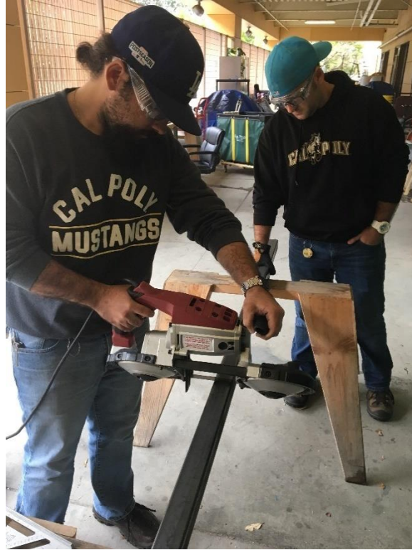
Figure 16. Cutting the Hollow Steel Tubing for the A-frame Legs Using A Portable Band Saw.
