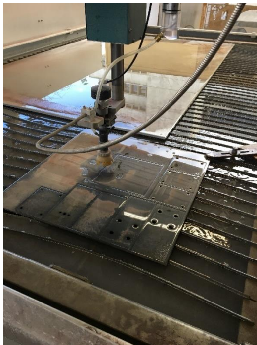
Figure 18. Water Jet on Gear Box Frame and Base Plates for the Caster Wheels.
