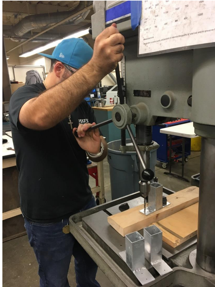
Figure 19. Drill Press Widening the Holes on the T-joints For Larger Bolts to Fasten the Support Bars to the A-frame.
