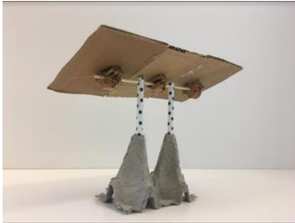
Figure 20. A concept model design for the tilt angle of the mount conducted during the concept prototyping. The panel rotates around the axial direction of the wooden stick with the rotation taking place at the straw/wooden intersection.
