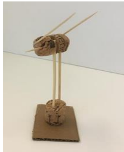
Figure 31. A concept model for the mount that has an azimuth angle adjuster at the top joint where the cork and tooth picks intersect, the two vertical stick members connected at each end with the bottom connection allowing for rotational adjustment, and the double prong stick to fasten the solar panels to.
