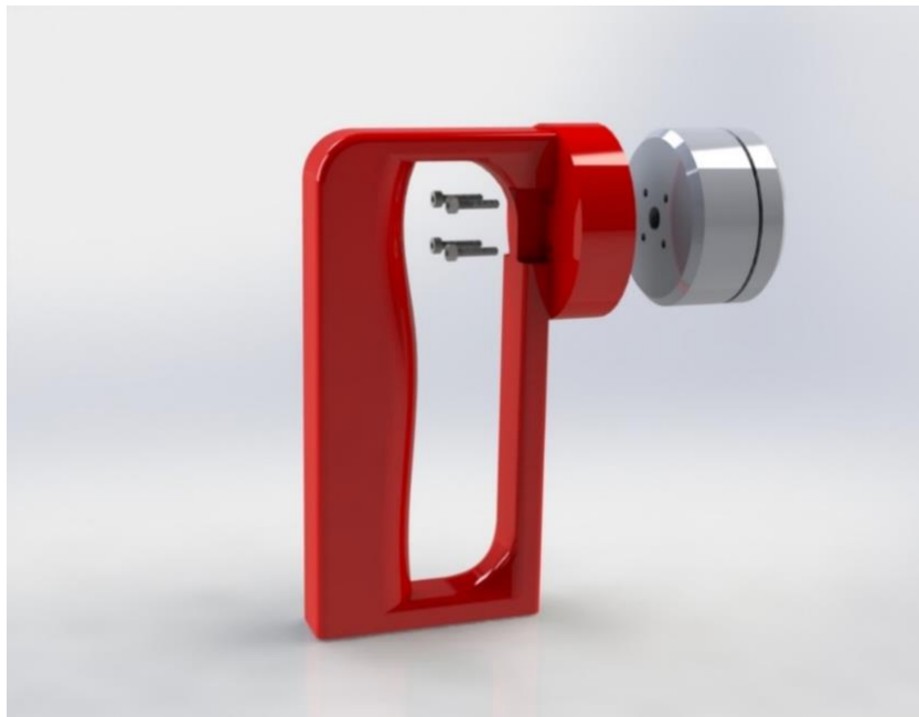
Figure 34: Attaching Motor to Handle
