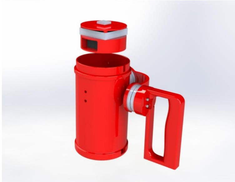
Figure 39: Placing Mounting Fixture Assembly in Mug Shell
