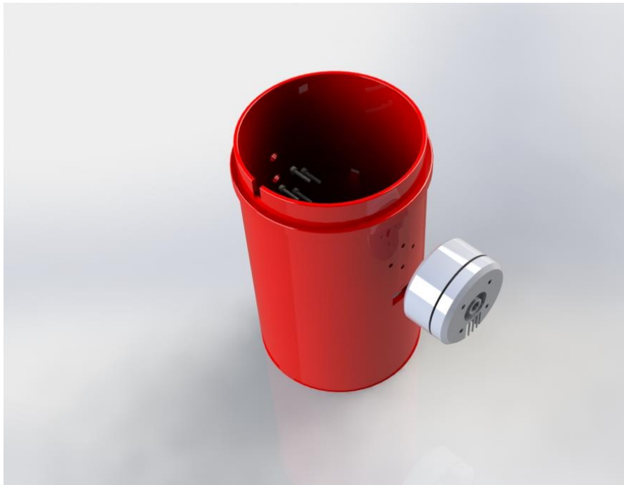
Figure 36: Attaching Motor to Mug Shell
