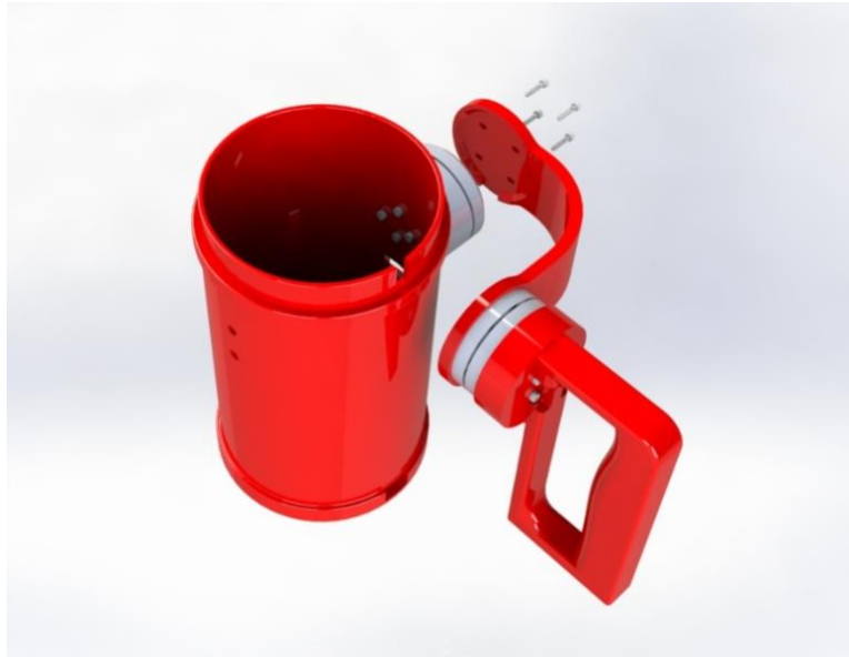
Figure 37: Attaching Bracket to Mug Shell
