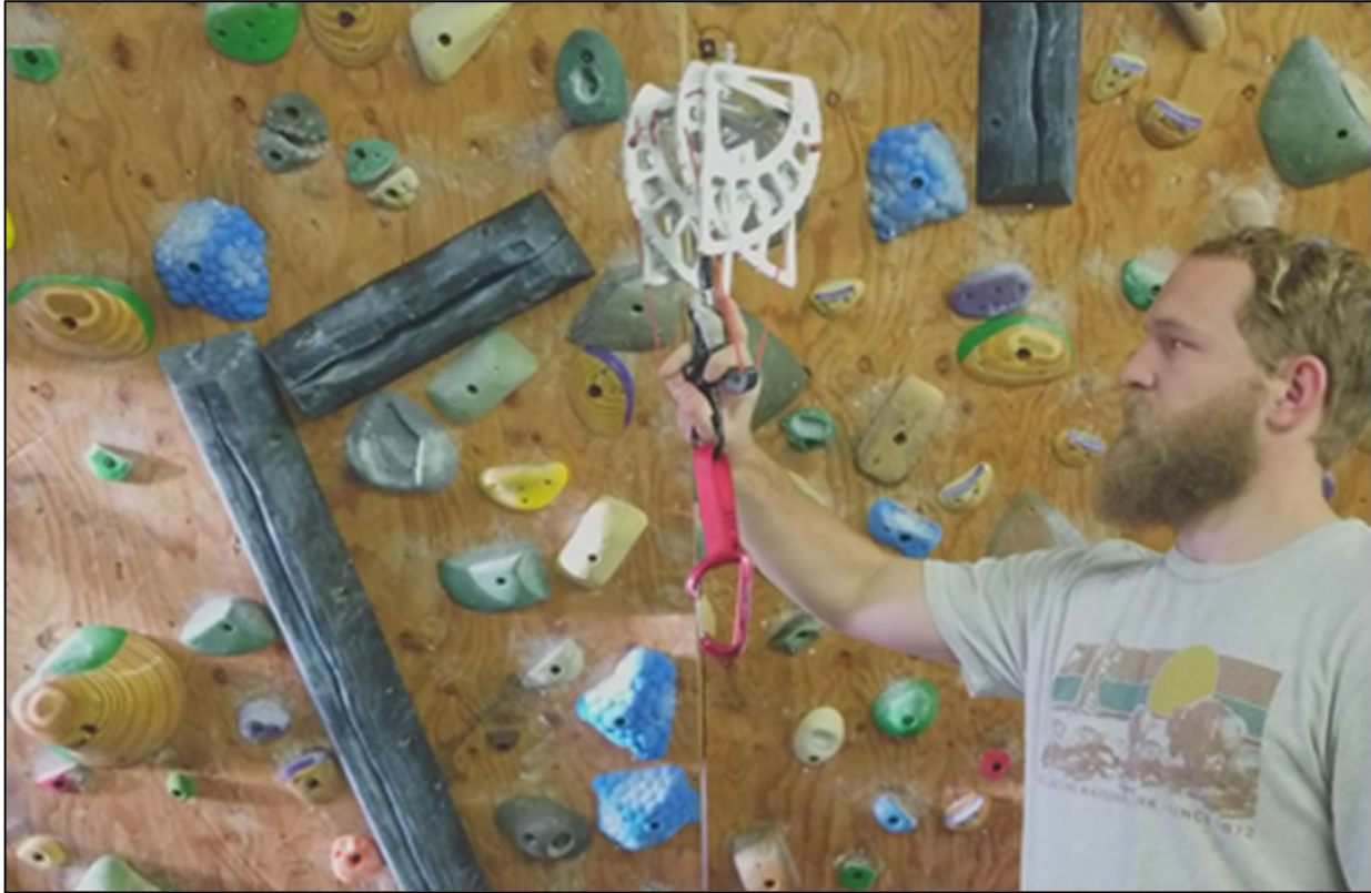
Figure 39. Testing that the stem does not buckle during the actuation of the cam.
