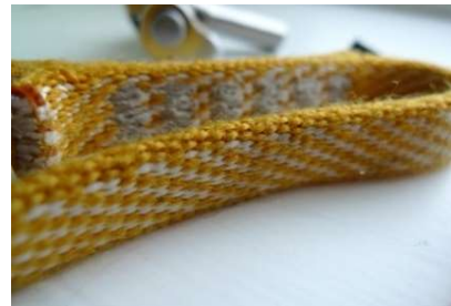
Some worn material in a sling.
