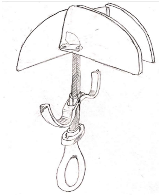
Figure 6. Drawing of Design A, which features a butterfly trigger, a pressed U stem, and a rotating collar lock.
