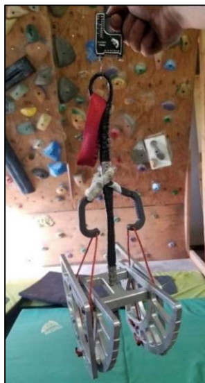
Figure 36. Weighing the cam. The weight is 1135 g.
