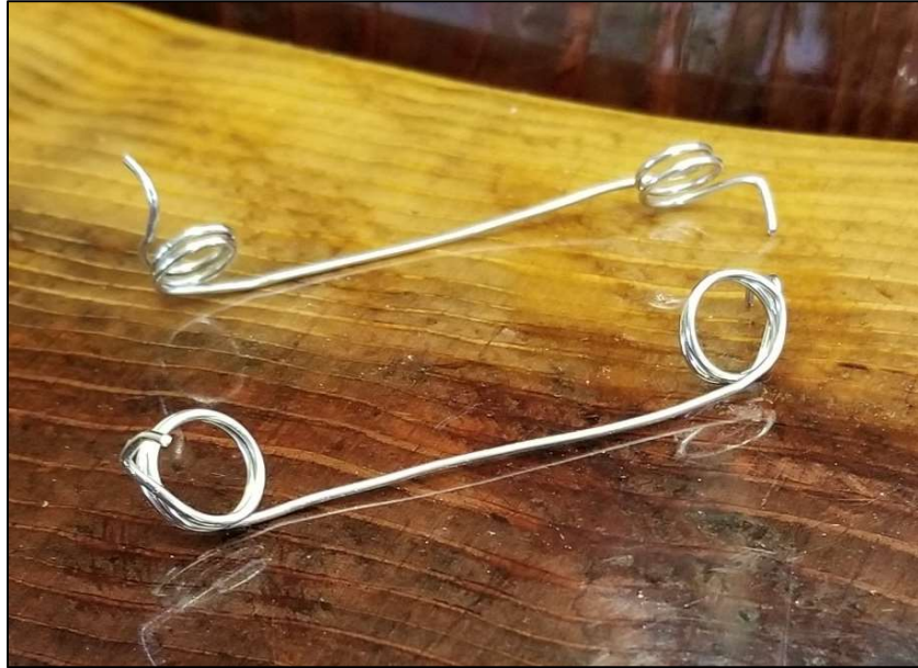
Figure 29. The finished torsional springs.
