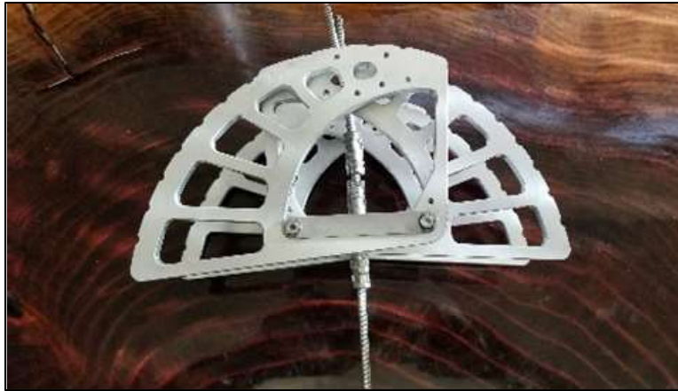
Figure 34. Lobes secured to the axles and carriage subassembly using snap rings.
