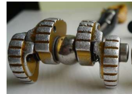
Worn down teeth on cam's lobes.
