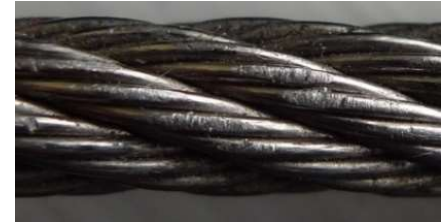
An example of worn wire cable.
