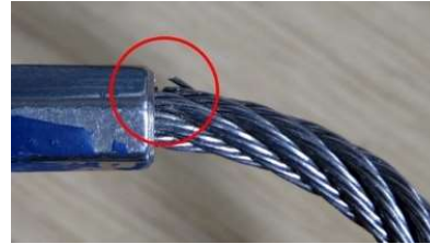
Fraying wire cable in stem.
