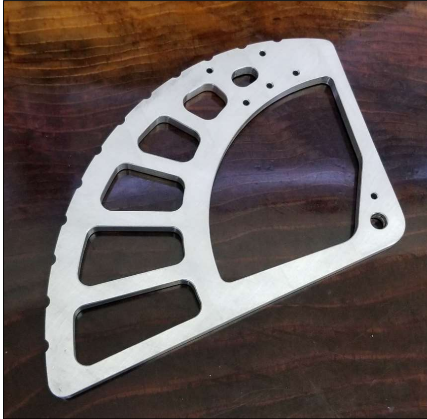
Figure 28. One of the finished lobes. We obtained this shape through extensive FEA.
