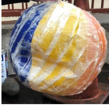
Figure 46. Deflated Beachball with Fiberglass Tape
