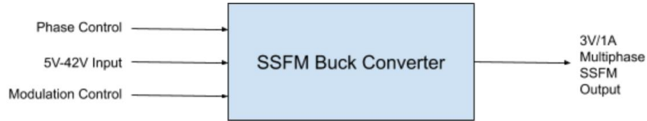
Figure 3-1: SSFM Multiphase Buck Converter Level 0 Functional Block Diagram
