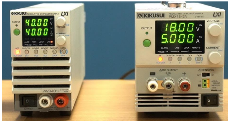
Figure 1-1: A 400W switching power supply (left) vs. a 90W linear power supply (right) [4].
