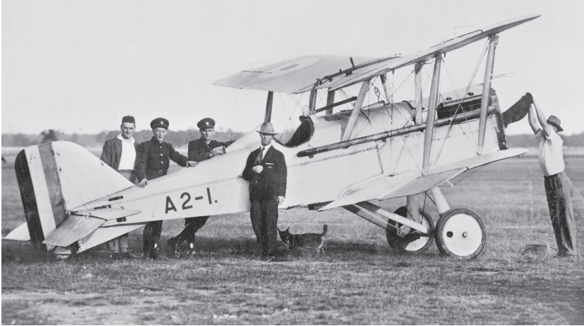
Figure 1.2. Royal Aircraft Factory S.E.5a #A2-1 at Yanakie, Victoria. This aircraft was one of 35 S.E.5as given to the RAAF by the British government as part of the 1920 Imperial Gift. The RAAF's leadership requested the S.E.5a over the Sopwith Snipe because the aircraft was more stable and easier to fly. (Photograph courtesy of the Australian War Memorial)
