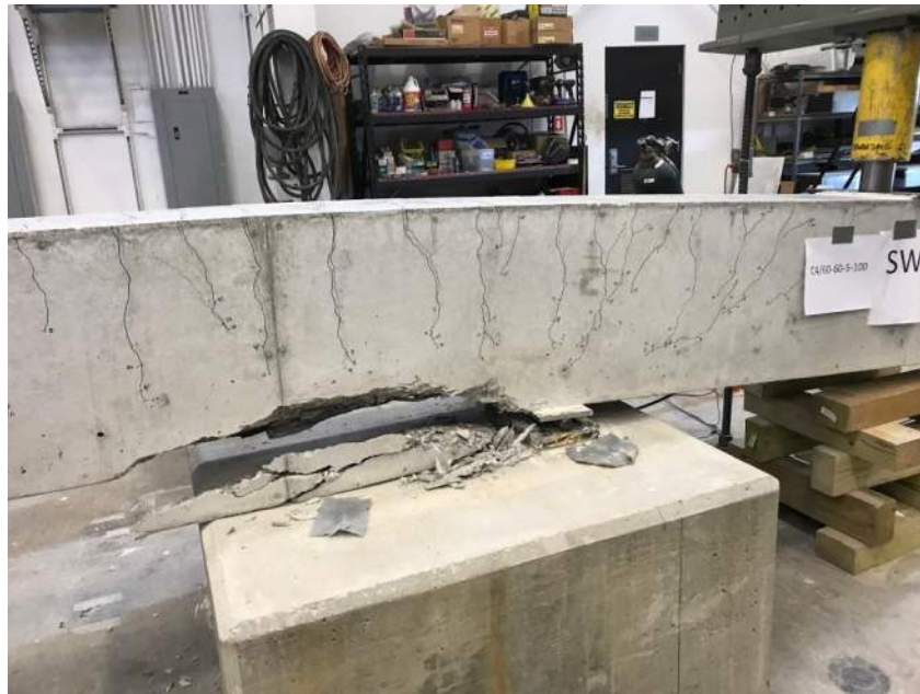
Figure 2.37: Flexural Failure (C4/60-60-5-100)
