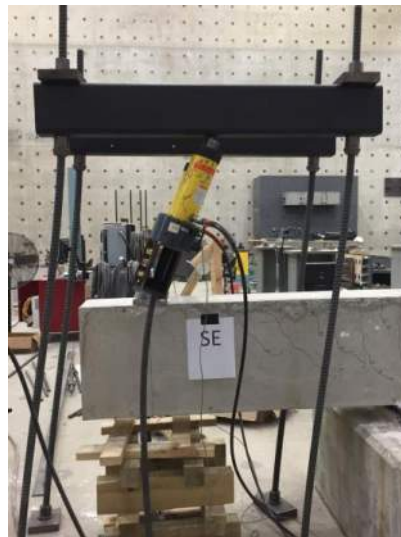
Figure 2.24: DYWIDAG Bars Yielding in Testing of U-80-5
