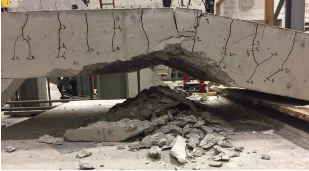
Figure 3.51: Final S-80-5 Failure – East Elevation
