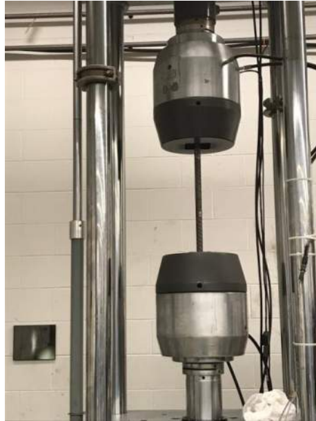
Figure 2.7: Testing of No. 8 Bars
