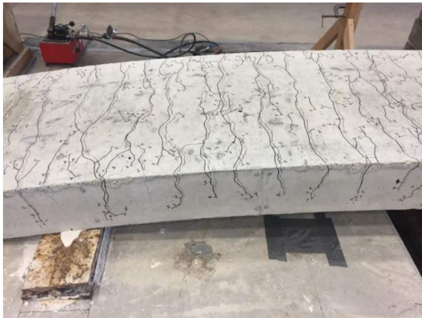
Figure 3.36: Typical Flexural Cracking – West Side and Tension Face (S-80-5)
