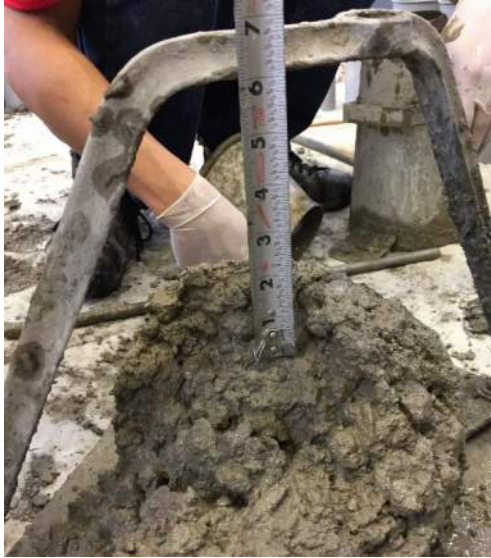
a) Slump Test
