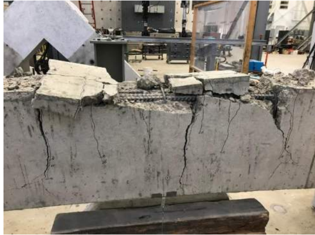
Figure 2.36: Typical Confined Specimen Failure (C3/60-40-5-100)
