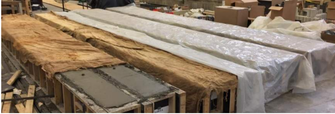
Figure 4.28: Series VI Moist Curing – Burlap Cover
