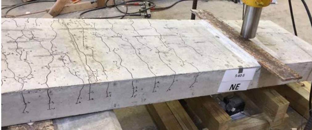
Figure 3.42: Post-Failure Shear Span Cracking (S-60-5)
