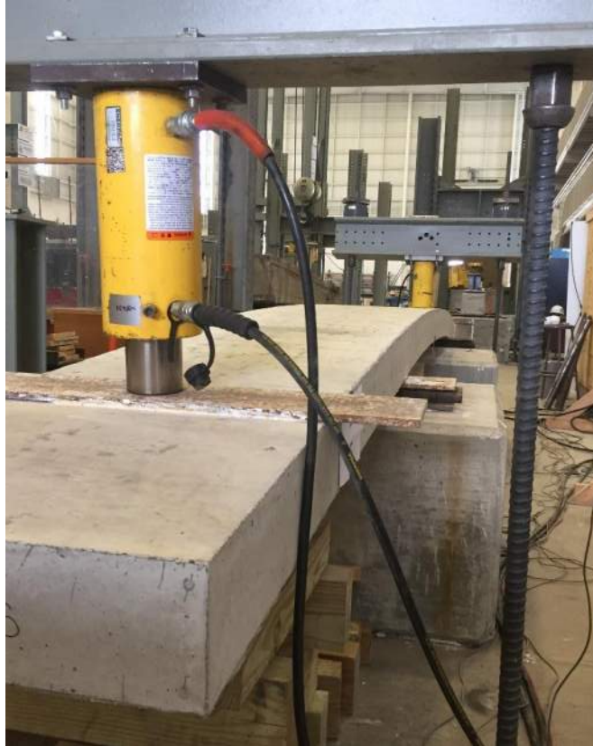
Figure 3.35: Slab Deformation during Testing (S-100-5)
