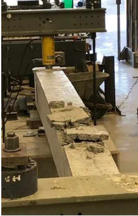
Figure 2.36: Typical Confined Specimen Failure (C3/60-40-5-100)
