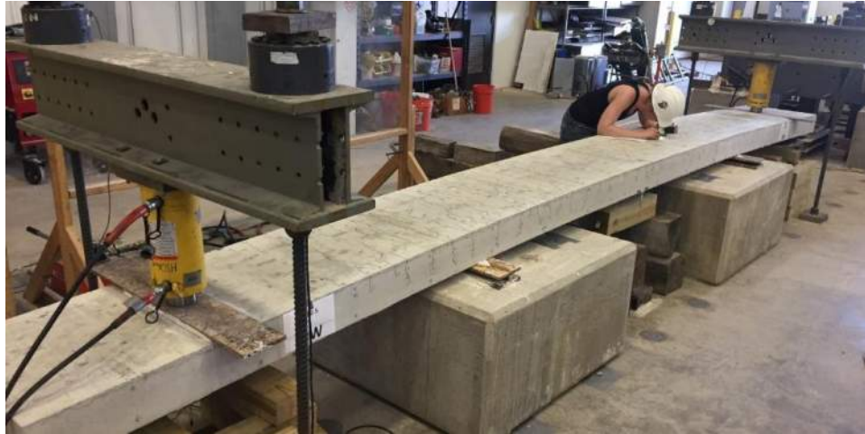
Figure 3.32: General Slab Test – Crack Mapping (S-80-5)
