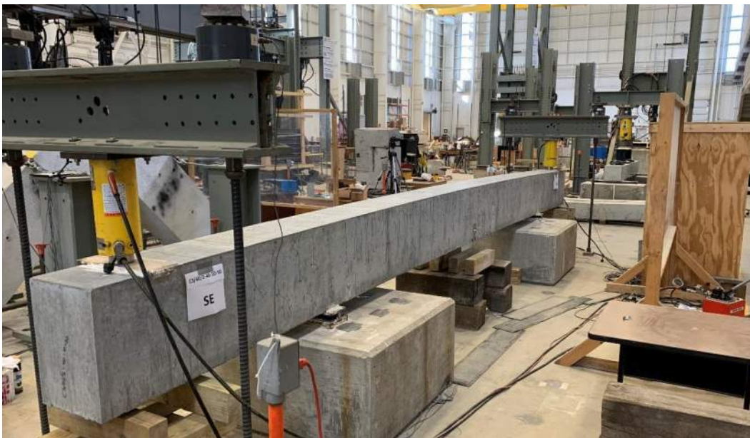
Figure 4.36: General Beam Test – Crack Mapping (C3/60/2-40-10-50)
