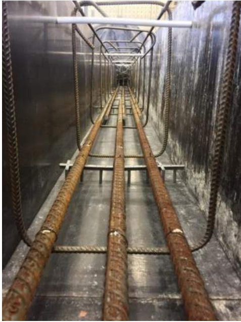
a) Confined Specimen
