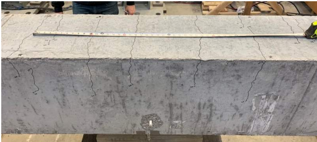
Figure 4.45: Transverse Flexural Cracking within Splice Region (C3/60/2-40-10-50)
