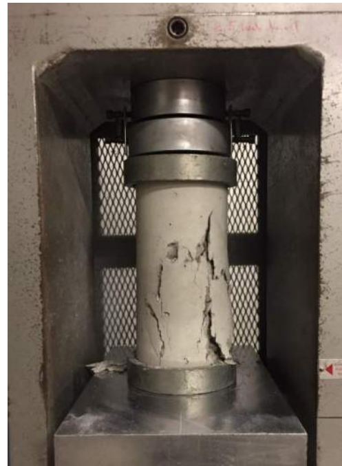
b) After Failure
