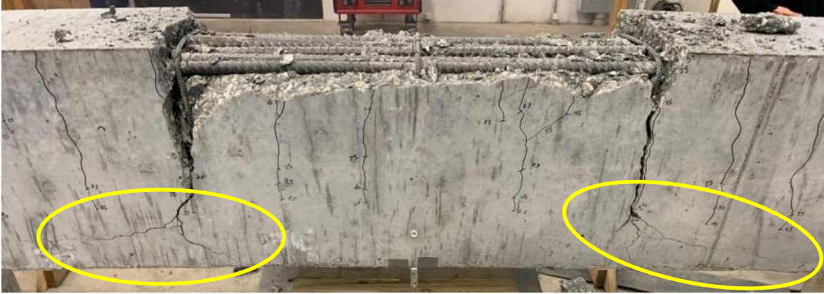
a) Full Splice at Failure
