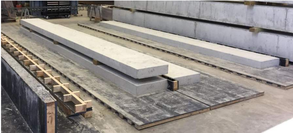
Figure 3.21: Series V Member Stacking and Storage
