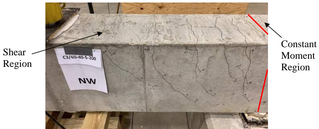
Figure 4.48: Shear Span – Late Testing (C3/60-40-5-200)
