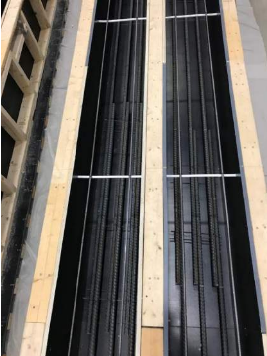
a) Unconfined Splice (Left: U-60-5, Right: U-40-5)
