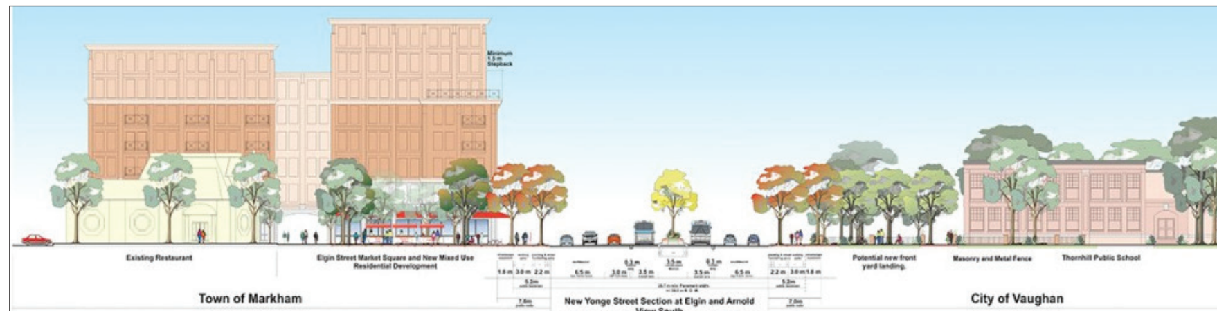
Thornhill Yonge Street Corridor Plan Section showing 6-8 storey mixed-use (left) and relocation of School frontyard parking.
