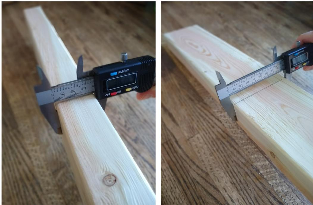
Fig. 4.2: Taking height and width measurements. Measurements were taken for height (left) and width (right) using digital calipers.
