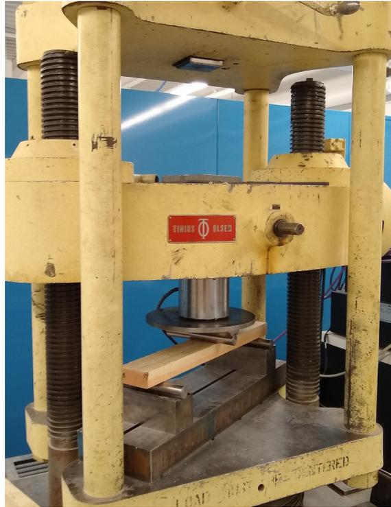
Fig. 4.3: Compression-tension universal testing machine. This machine was used to apply a midspan point load to measure the modulus of rupture.
