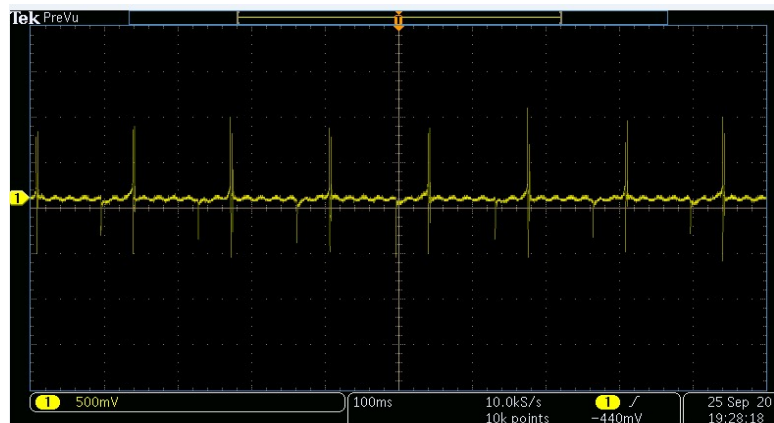
Figure 4. Piezoelectric analysis of the PVDF nanofiber membrane at a cyclic applied force of 5 N and at a rate of 5 Hz. The shown y-axis presents electric voltage (in volts) and the x-axis is the time (in seconds).
