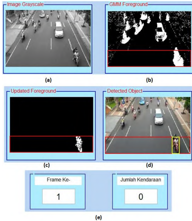
Gambar 5.6: Contoh proses counting pada input video ketiga (a)citra grayscale (b)foreground hasil GMM (c)updated foreground (d)tracking dan counting (e)indeks frame dan hasil counting .
