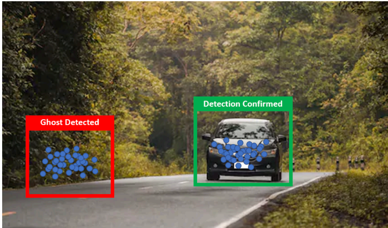
Figure 2. Ideal Output of Noised Removed Point Cloud
