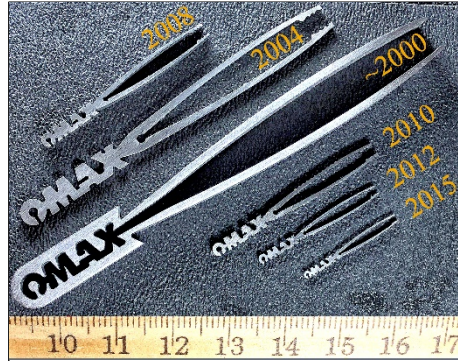
Figure 4. Progress toward AWJ micromachining - tweezers
