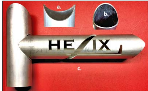
Figure 17. AWJ-cut “fish mouth” weld joints using combined operation of Rotary Axis and A-Jet
