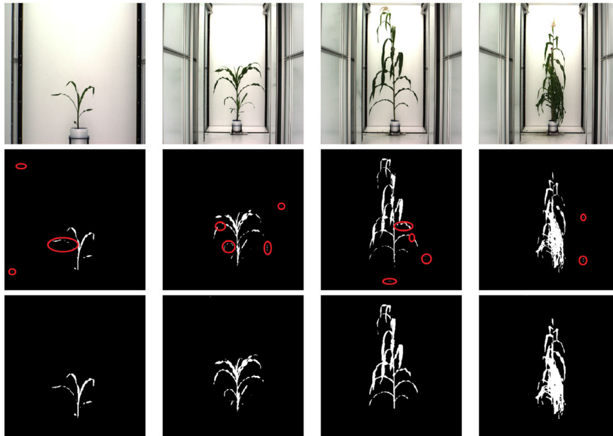
FIGURE 6 A comparison of double-criteria thresholding (in the middle row) and segmentation using a neural network (in the bottom row) trained on the full neighborhood dataset. Areas marked in red highlight are where the neural network outperformed double-criteria thresholding
