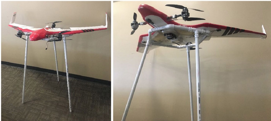
Fig. 10 Top and bottom view photos of a FireFLY6 PRO fixed wing UAS atop the holding tripod
