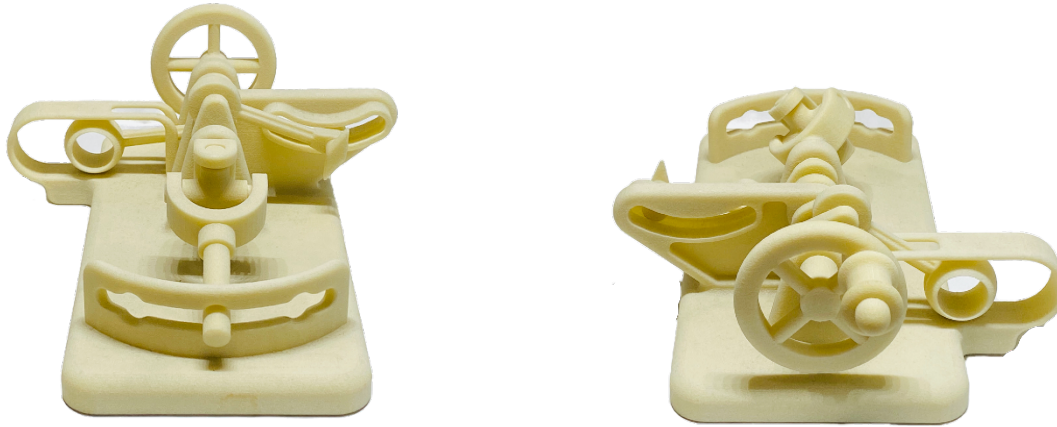
Figure 2.4: Single PBF Nylon Print
