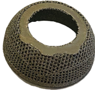
Figure 2.13: Partial Print of Acetabular Hip Replacement Cup
