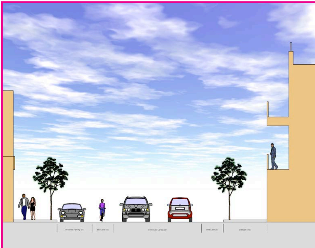
Figure 26: Haven Avenue cross section.
