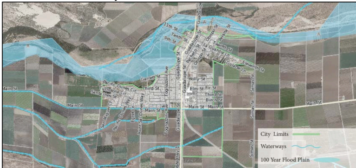
FIGURE 49. AREAS SUBJECT TO 100-YEAR FLOOD INUNDATION
