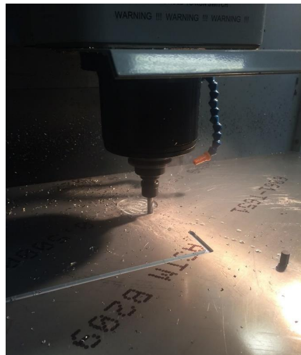
Figure 62: The 4" fan holes being end-milled and the L-shaped datum slot
