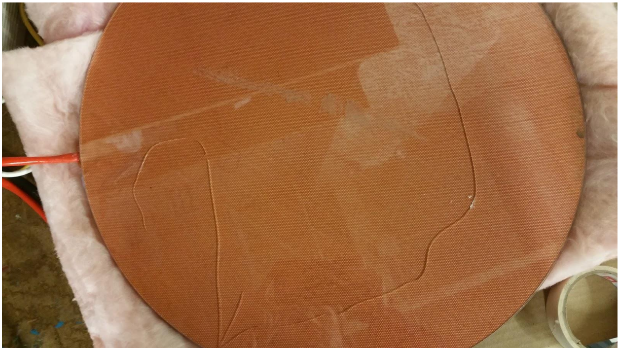
Figure 65: Cracked soda lime glass
