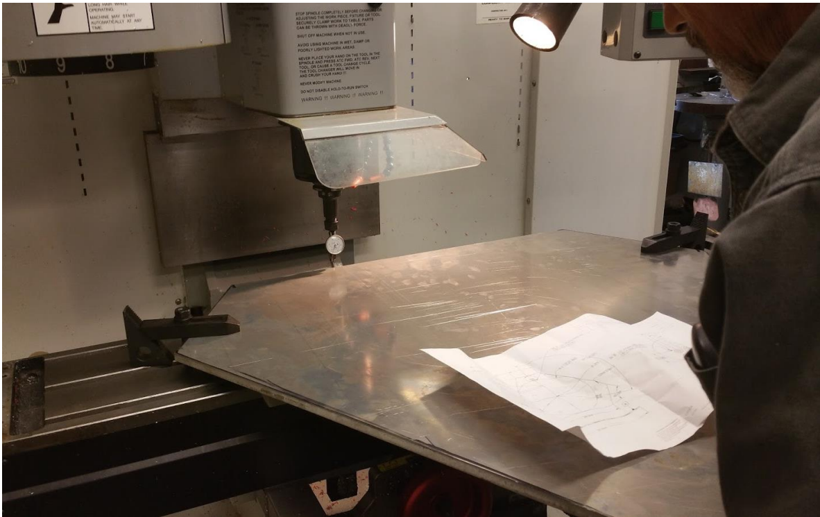
Figure 59: Aligning and clamping the aluminum plate
