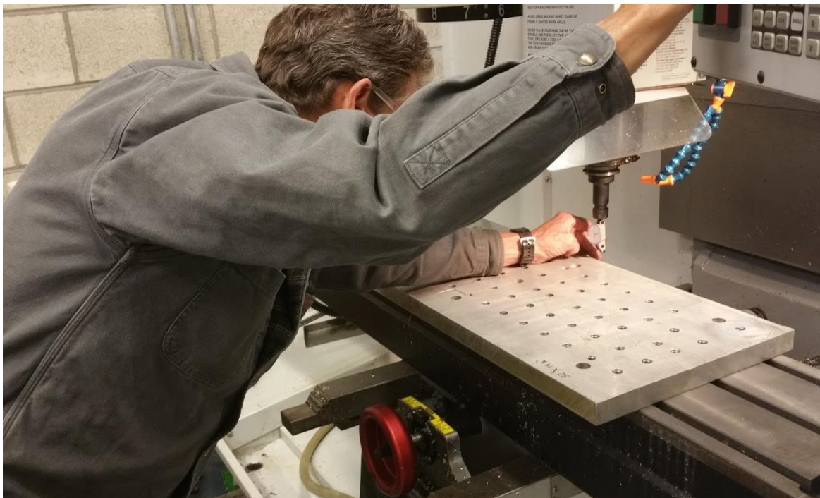
Figure 58: Ladd Caine aligning the back edge of the underplate
