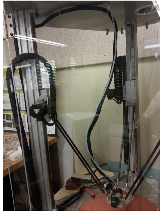
Figure 75: Extruder wiring in shrink tubing
