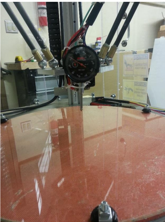
Figure 80: Dial indicator zip-tied to platform
