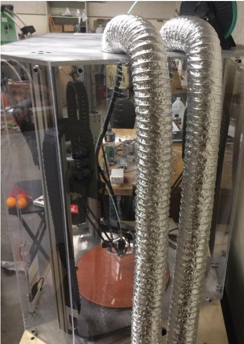
Figure 70: 4" ducting as seen from above
