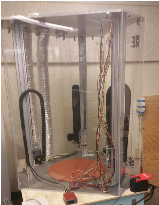
Figure 74: Loose extruder wiring
