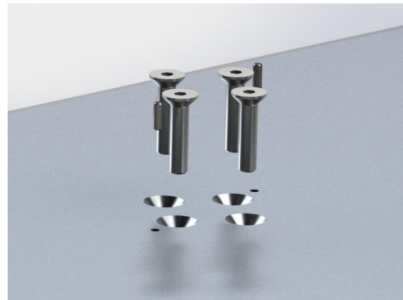
Figure 48: Hole pattern for T-slot and plates
