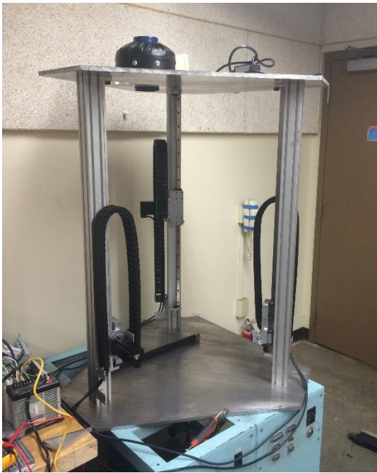
Figure 69: Bell-Everman linear slides attached to top and bottom plates
