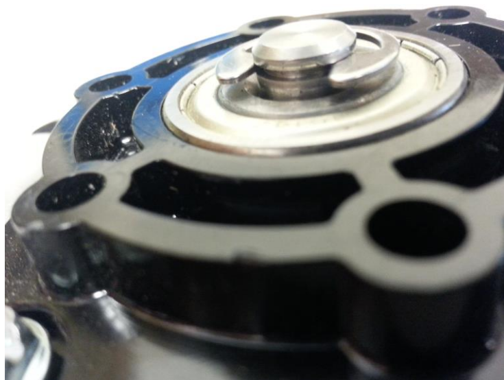
Figure 54. Wheel shaft with retaining ring after being press fit into bearing.
