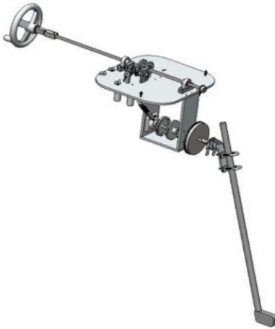
Figure 8: Computer model of the Universal Play Frame golf attachment. [2]
