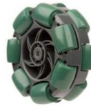
Figure 22: Omni-directional wheel used on VEX robots. [20]
