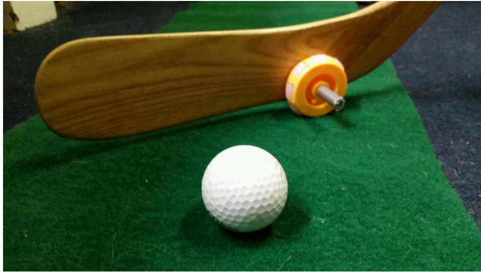
Figure 30. Preliminary testing of 2.75 inch diameter omniwheels.
