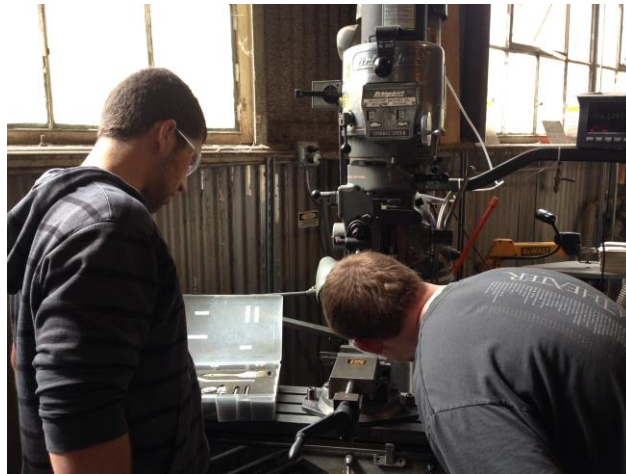
Figure 44. Chris and Joseph drilling the 3/16" holes along the shaft.
