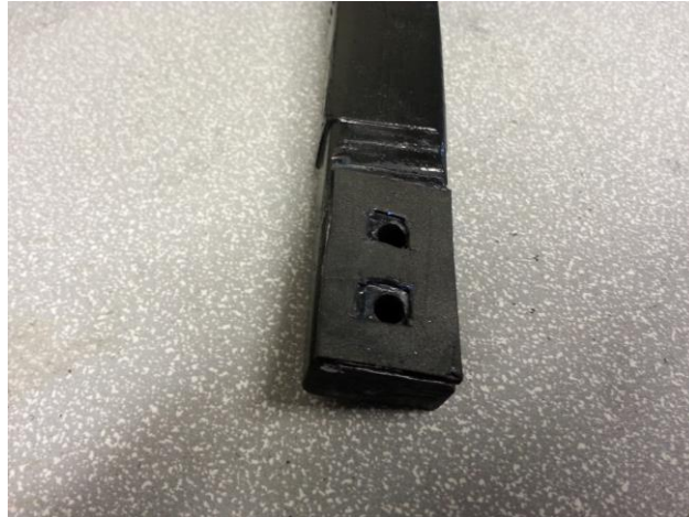
Figure 57. The top of the putter attachment with the two pin holes and the added foam for a tight fit.
