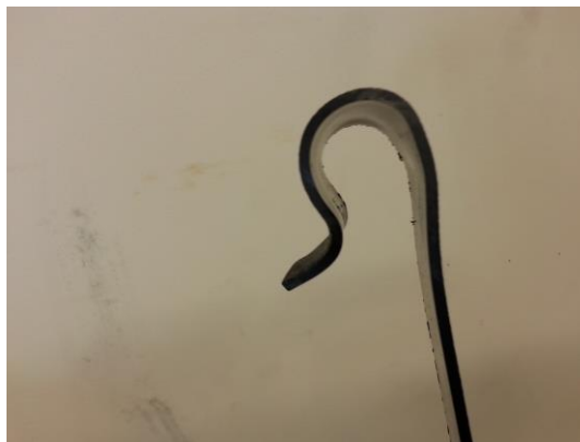
Figure 60. The lip shape that was heat-formed over conduit.
