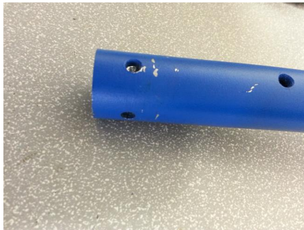
Figure 47. The main shaft showing the original holes and the redrilled holes.
