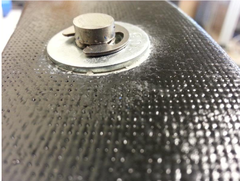
Figure 55. The end of the shaft that was passed through the blade.
