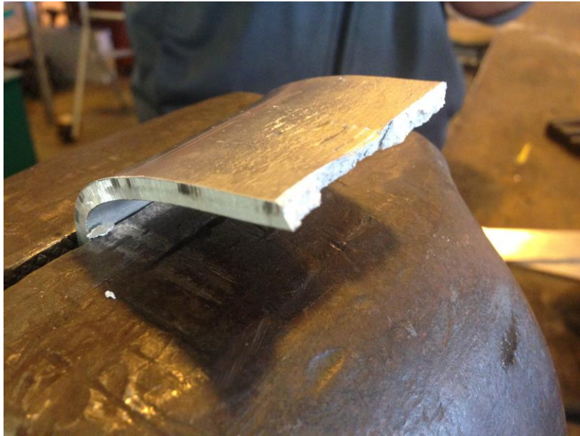
Figure 53. The .16" plate after snapping while being bent.
