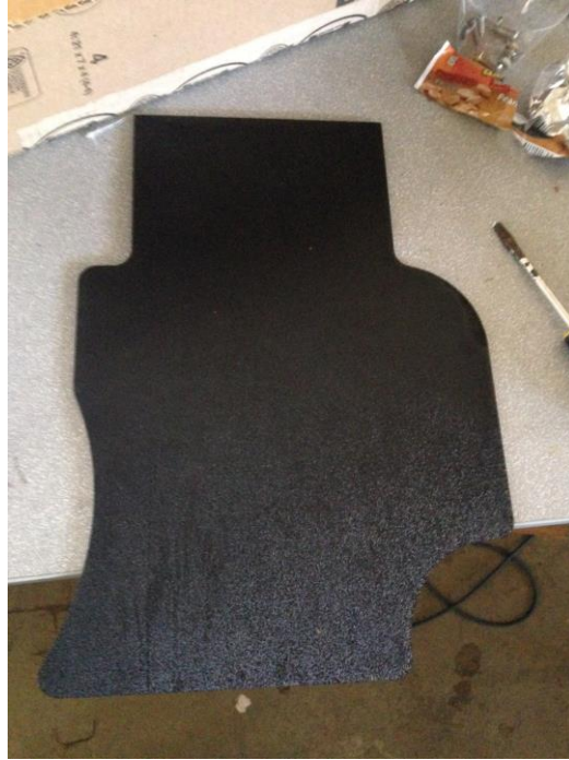
Figure 59. A kickball guard after being laser cut.
