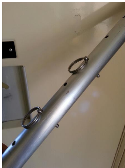
Figure 45. Main shaft with holes drilled along it and pins in two of the holes.
