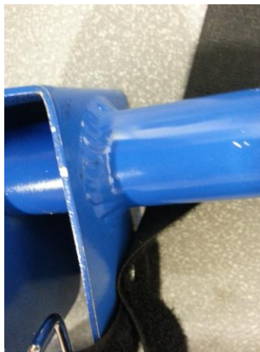
Figure 51. U-bracket welded onto the main shaft.
