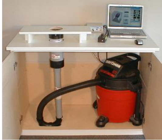
Figure 5. Example of a basic flow bench created using a shop vac (Flow Performance, 2015).
