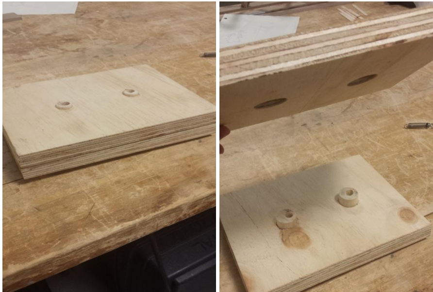
Figure 11. Wooden model demonstrating the removable fixture concept. The top board represents the blade fixture with counter bored bottom connections. The bottom board represents the table interface with extruded connections to fit into the bores on the fixture.
