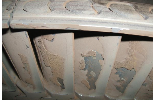
Figure 2. An example of deposits on used turbine blades (Janikowski, 2011)
