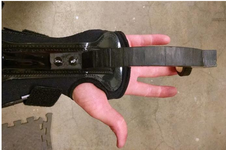
Figure 48: Bottom view of underhand mount and wrist guard attachment
