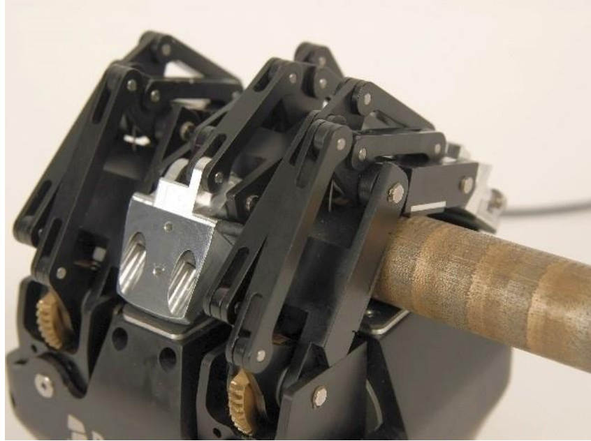
Figure 2: Robotiq 3-Finger Adaptive Gripper holding round stock (Robotiq, 2014)
