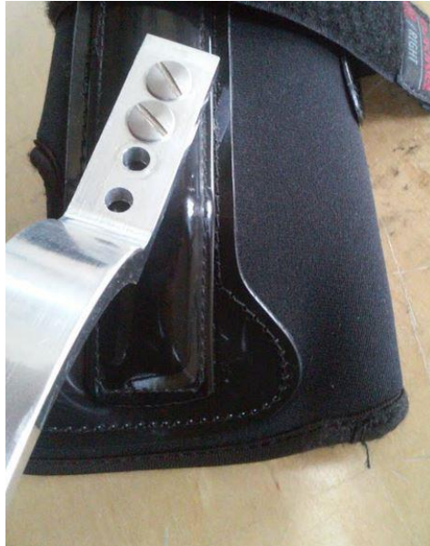
Figure 50: Underhand mount with 15.5 degree offset and optimized length of 5.2 inches
