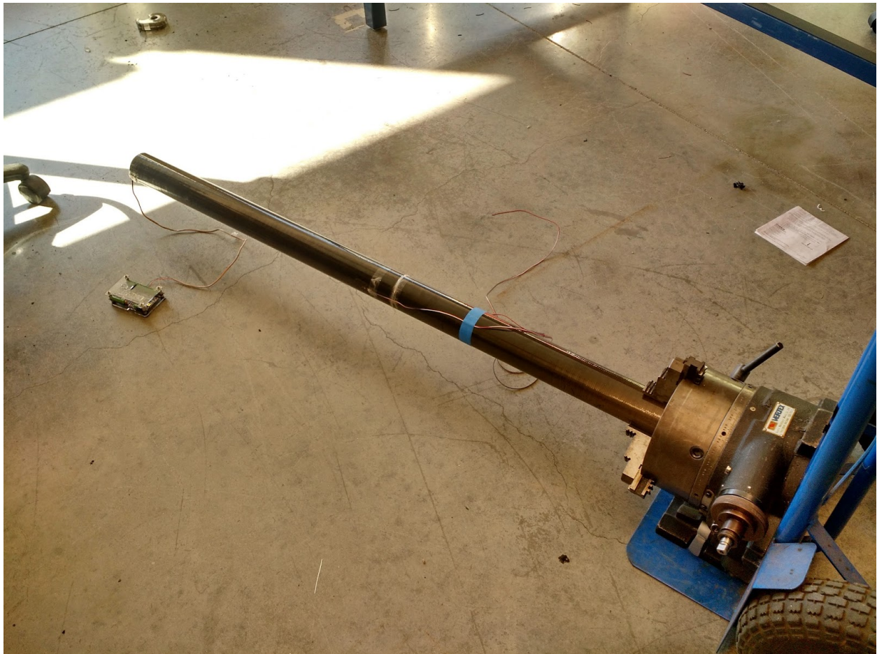
Figure 3. Depiction of the cantilever vibration test performed on the carbon fiber tube.
