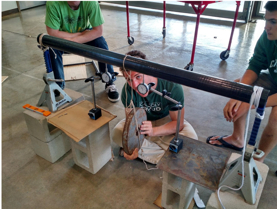
Figure 1. Previous testing run by the Electric Commuter Multicopter senior project team which estimated the flexural modulus of a carbon fiber tube.
