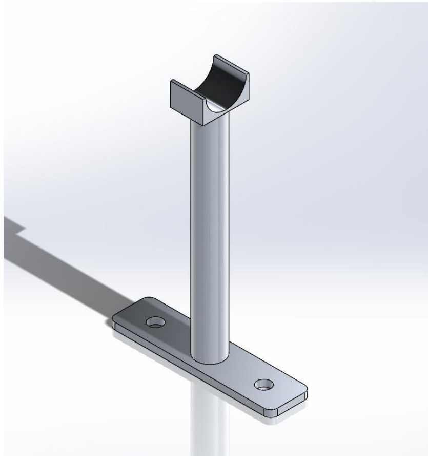
Figure 83: Joystick stand used to lock down the joystick fork for operational use
