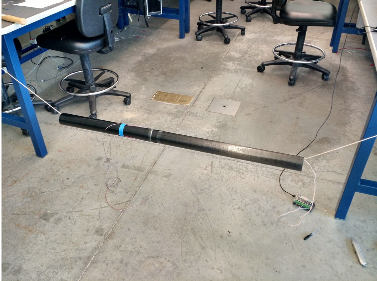
Figure 4. Free-free test apparatus used for vibration testing the carbon fiber tube.
