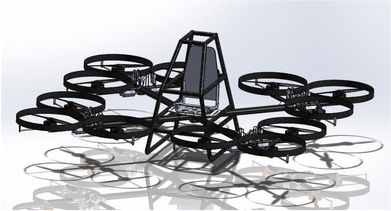
Figure 86: One possible roll cage design constructed from carbon fiber added to the final multicopter structure.
