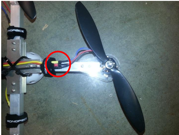
Figure 2a(Left) Black, CW-rotating motor wiring configuration
