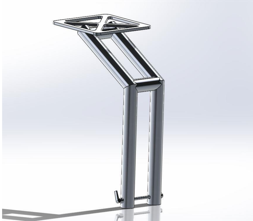
Figure 82: Solid model of the joystick fork, which allows the user to rotate the joystick plate away from the user during entry and re-entry.
