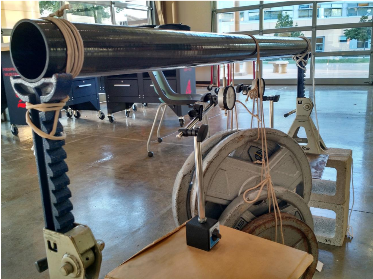
Figure 87: Experimental apparatus for the three-point bend test. Note the pair of dial indicators on either side of the load.
