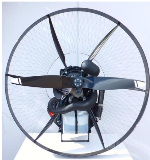
Figure 7: Scout Paramotors' device to counter the angular momentum of the paramotor.
