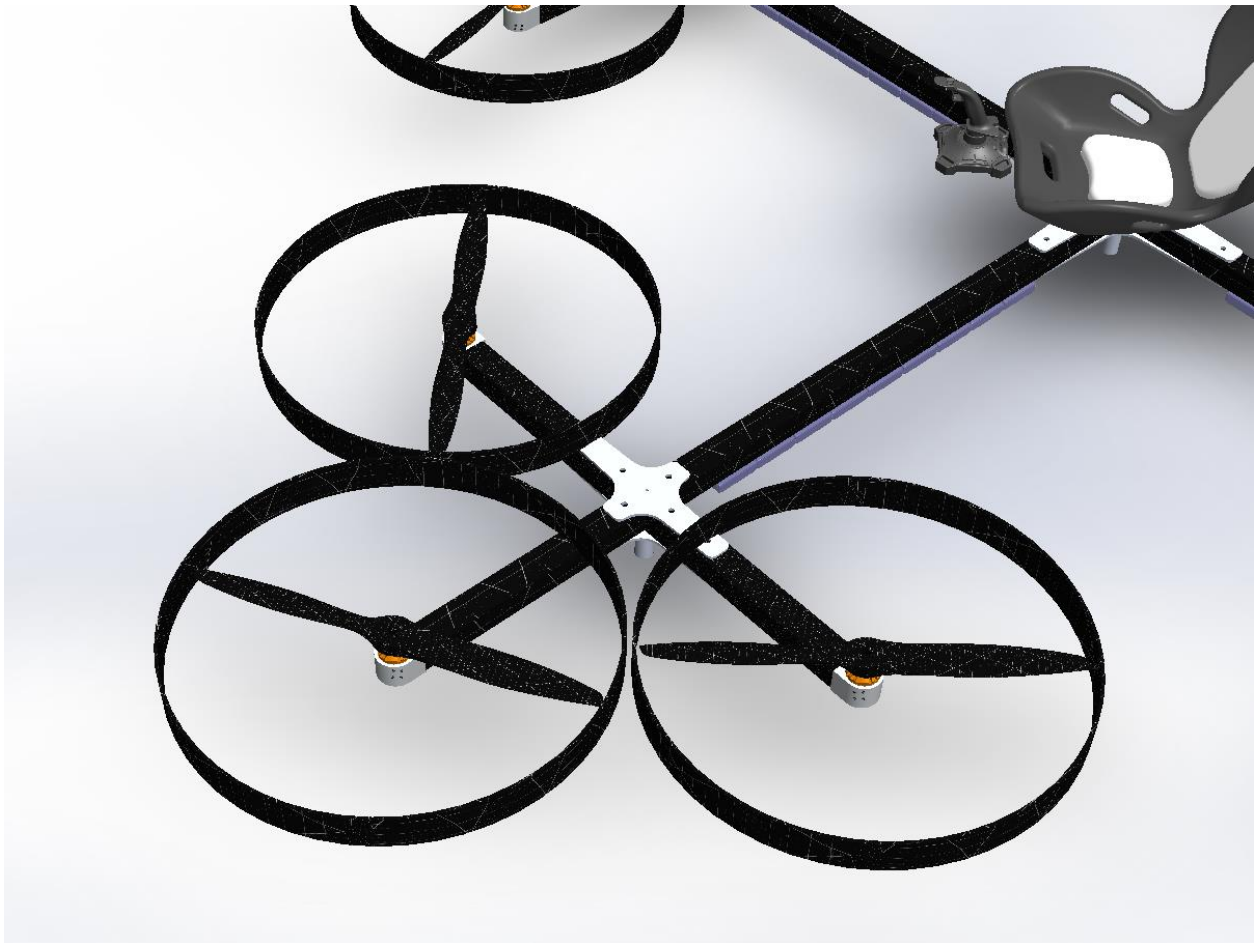
Figure 25: Grouping of propellers on each arm in preliminary design.
