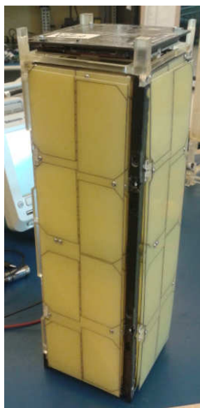
Figure 4.3 Printed Prototype of Tesseract Structure.
