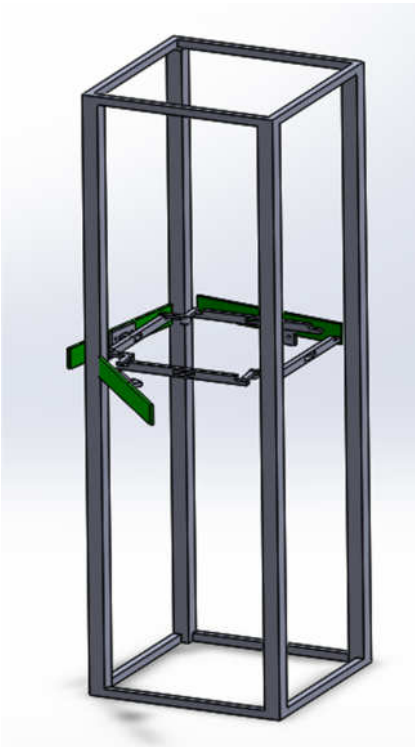
Figure 3.12 Concept CAD model of "Bar Linkage without Center Plate" Release Mechanism Concept
