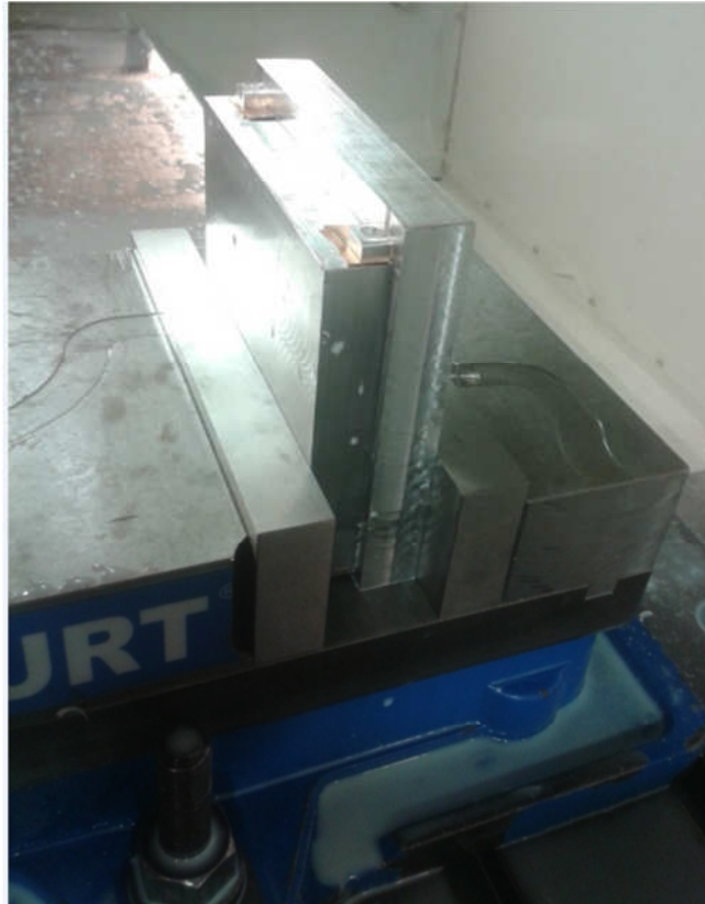
Figure 5.5 Top hat with bronze shims for spacing.
