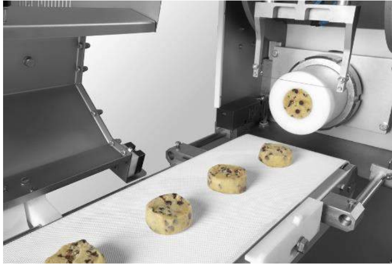
Figure 1: Still shot of the Vemag Reiser cookie dough extruding machine
