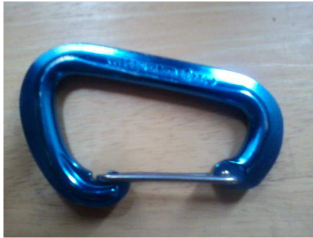
Figure 33: The rock climbing carabiner used for dough testing
