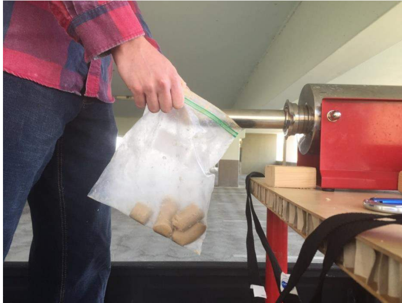
Figure 35: Dough extruded from the sausage press is collected in a bag of known weight
