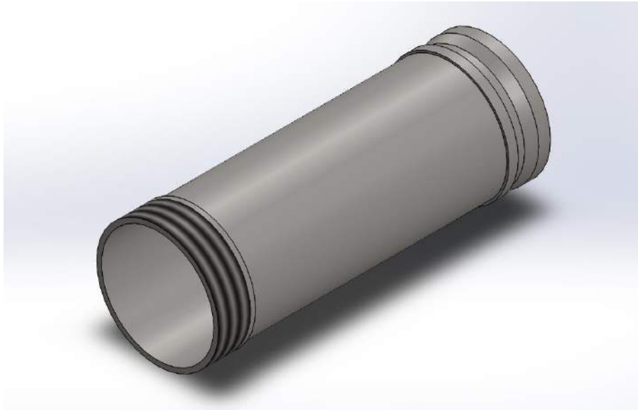
Figure 21: Isometric rendering of the cylinder (201) showing threads and back lip
