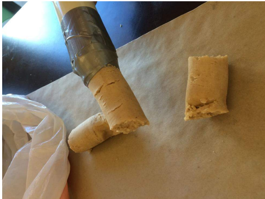
Figure 40: The first successful contraction and extrusion test
