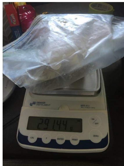
Figure 36: Extruded dough being weighed during testing
