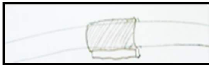
Figure 35. Cable Guides with Collar Attachment
