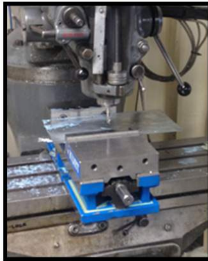
Figure 138. Milling Spool Mounting Plate
