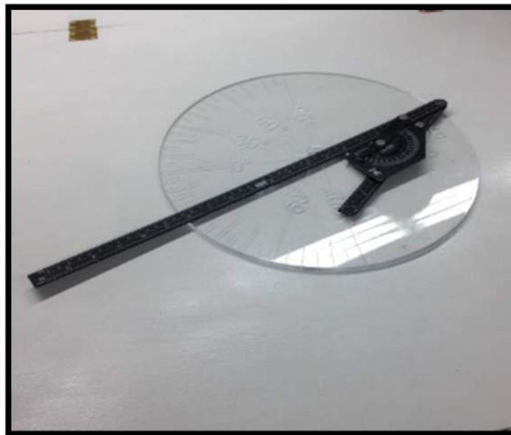
Figure 170. Angle Accuracy Test Setup
