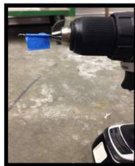
Figure 137. Hole-Depth Marking Method
