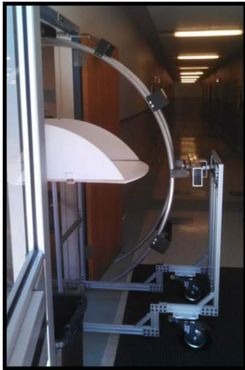
Figure 168. Heliodon in a Doorway
