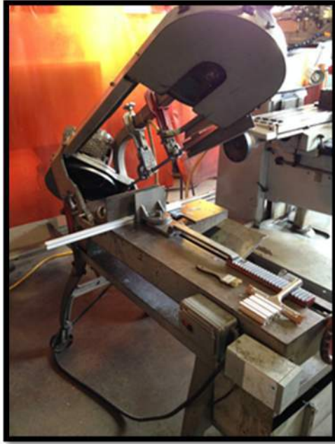
Figure 132. Horizontal Band Saw Cutting T-Slot
