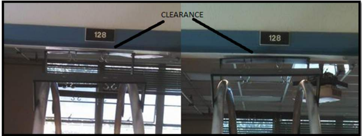
Figure 169. Heliodon Top Bracket Clearance
