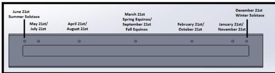
Figure 64. Slot Holes for Various Times of the Year
