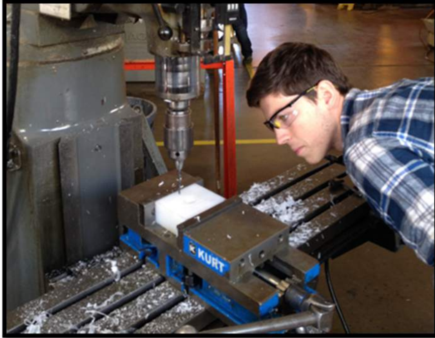
Figure 148. Drilling Front and Top Holes into UHMW Slider
