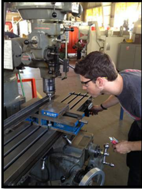
Figure 142. Attempting to Mill Steel Angle
