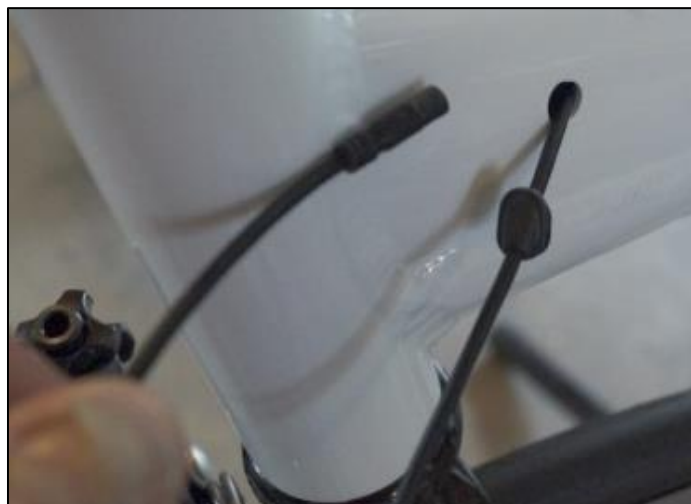
Figure 6. Boss in the bicycle frame
