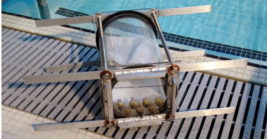
Figure 21. Revision 1 of the watertight vessel, fully assembled.
