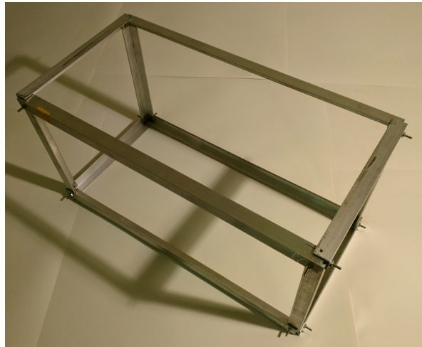
Figure 13. Assembled aluminum chassis.
