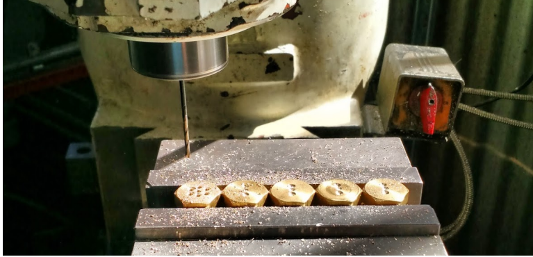
Figure 16. Second attempt at fabricating thru hull connectors.
