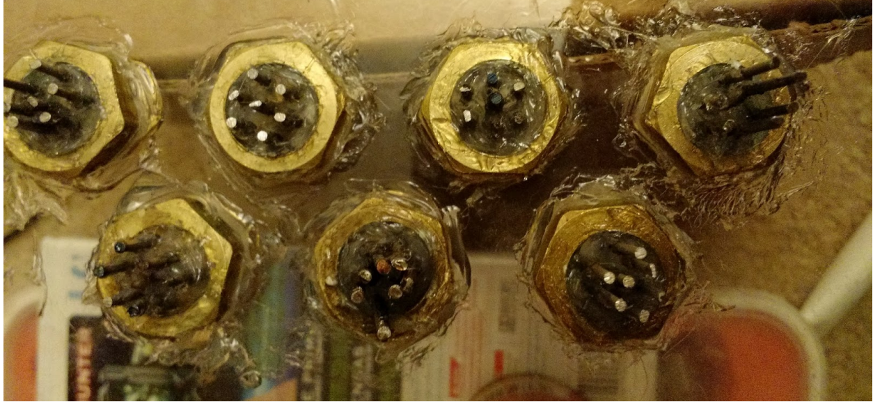
Figure 17. Epoxy drying on the thru hull connectors.
