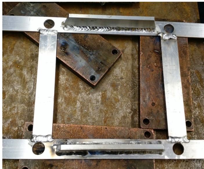
Figure 19. Fully fabricated vessel mount.
