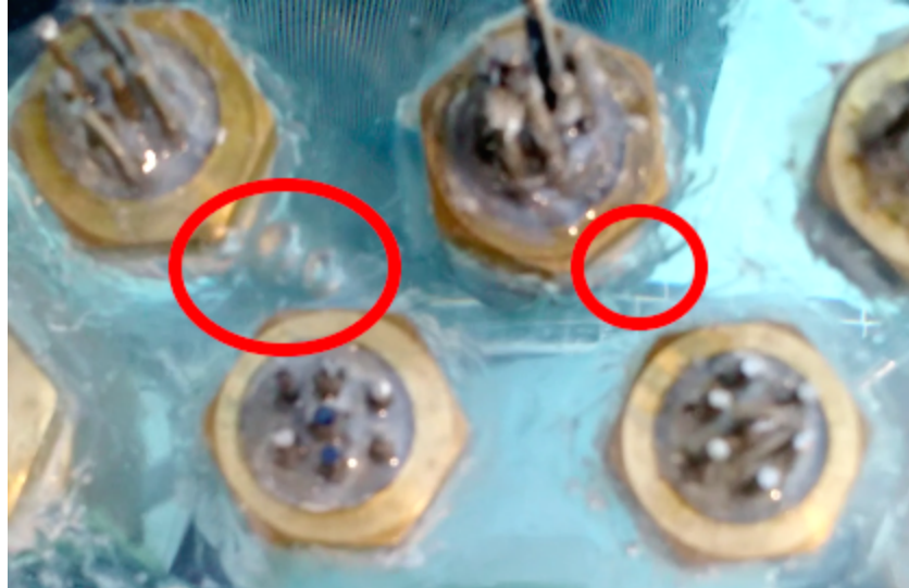
Figure 23. Air bubbles leaking from thru hull connectors on Revision 1.
