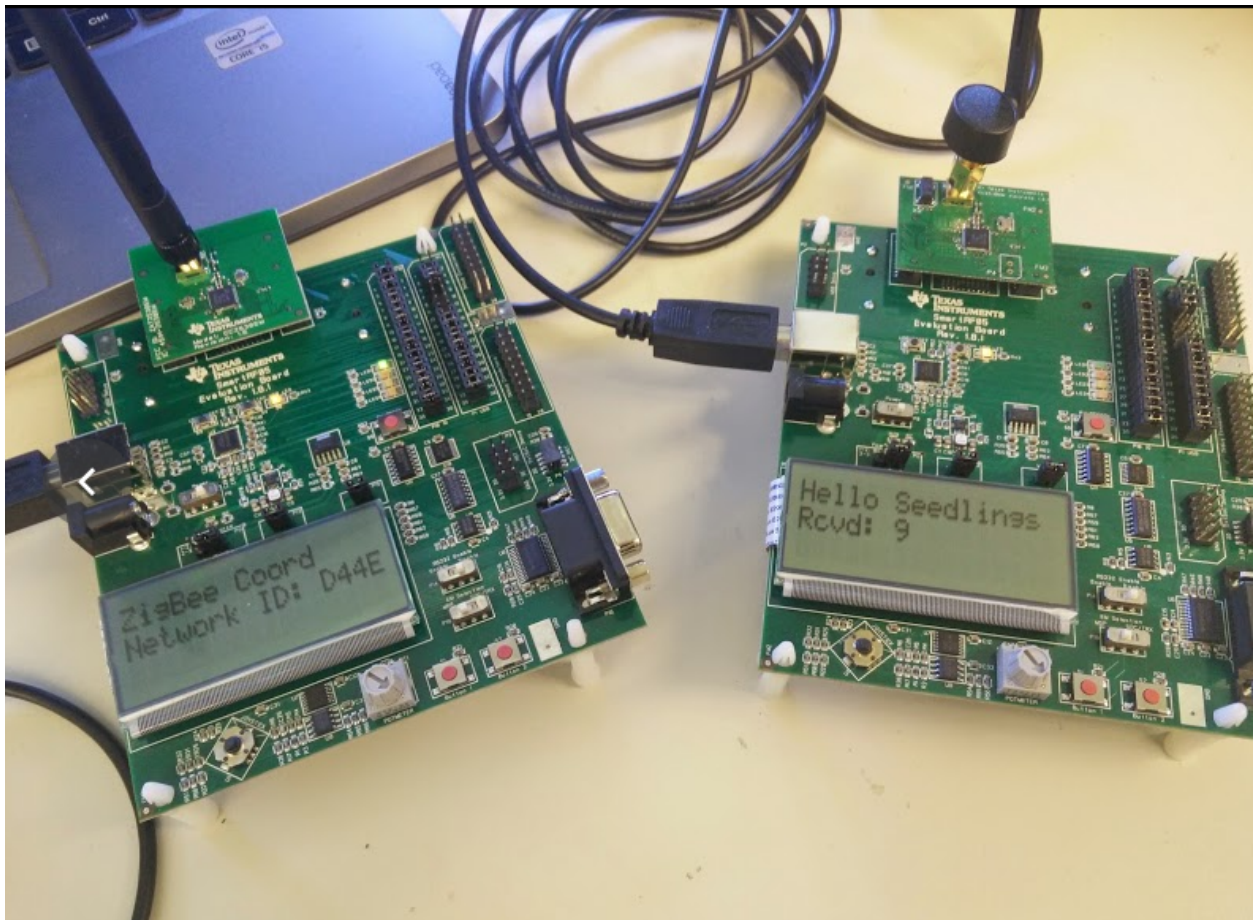
Figure 5a: Zigbee coordinator sending data to router
