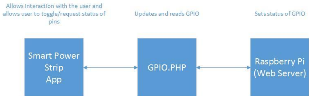
Figure 11: Web Server Block Diagram
