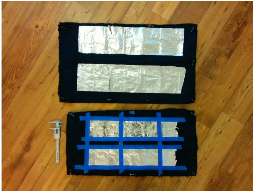
Figure 5 Prototype Bed Sensor Pads. Calipers Provided for Scale.
