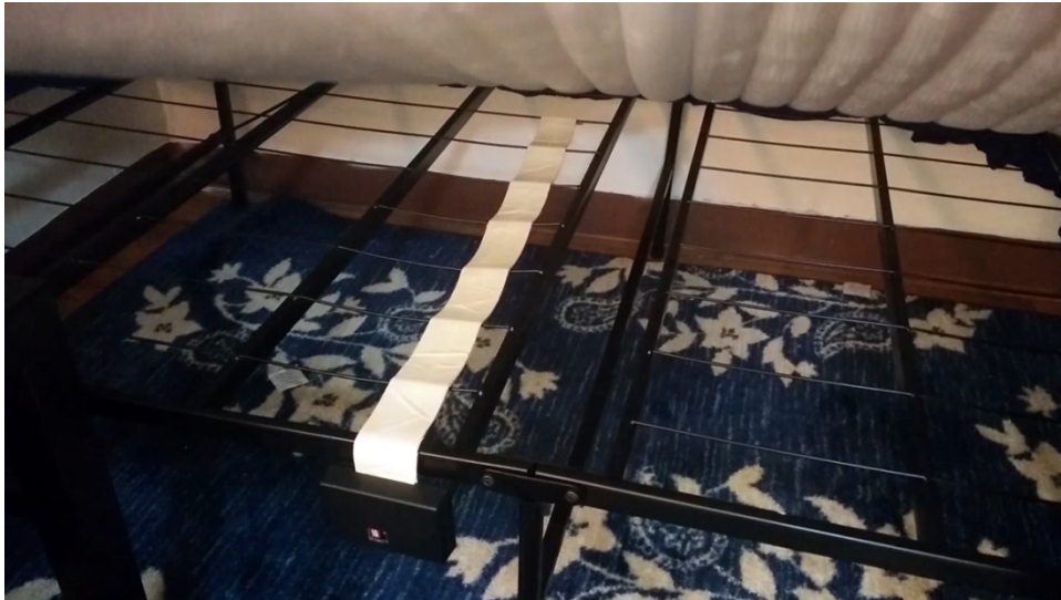
Figure 14 Placing the Sensor Under a Mattress
