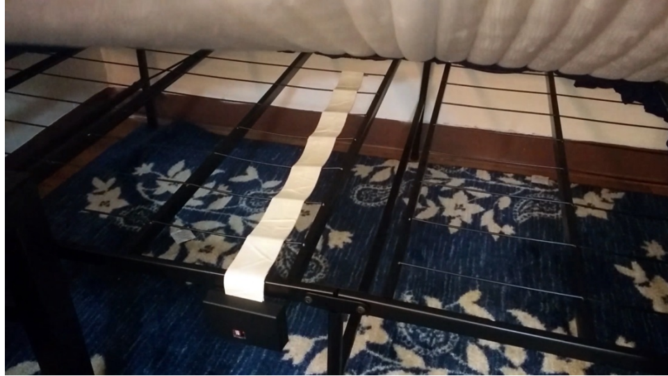
Figure 8 Strap Sensor Under a Mattress
