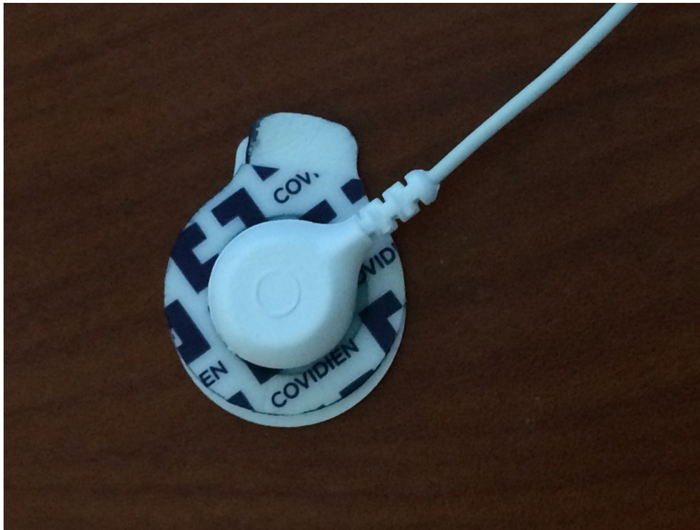
Figure 12: Sample electrode used to receive EMG signals
