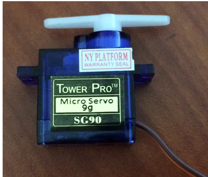
Figure 14: Servomotor used to control the string movement
