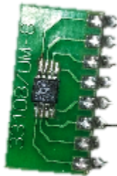
Figure 5-1: SMD LT6105 Soldered onto Breakout Board
