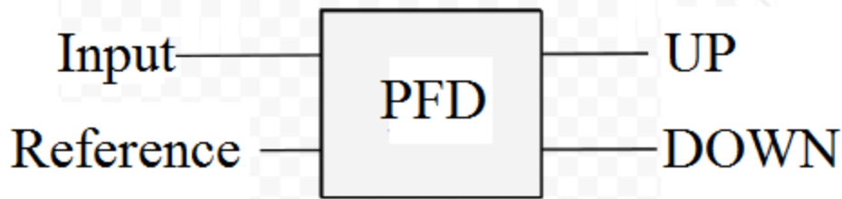
Figure 5: PFD Highest Level Block Diagram
