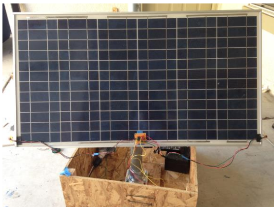
Figure 13 Photo of Sensors Mounted onto Solar Panel
